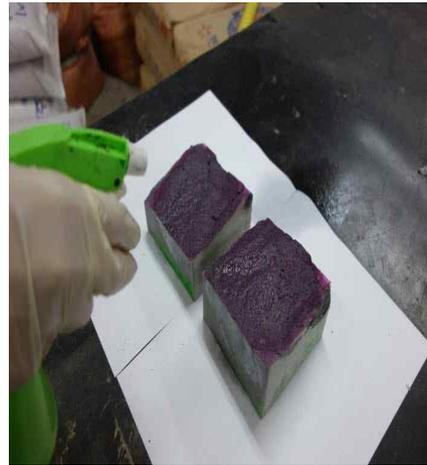
Fig. 3. Photos of carbonation resistance test of concrete with modified sulfur.
