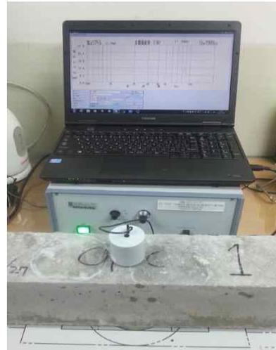
Fig. 4. Photos of rapid freezing and thawing test. (a) Test chamber, (b) Measuring dynamic elastic modulus of specimen
