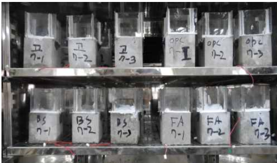
Fig. 8. Photo of ponding freeze-thaw test chamber.
