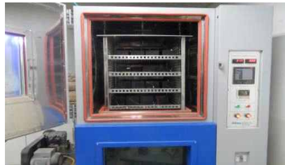
Fig. 5. Photo of freeze-thaw test chamber.
