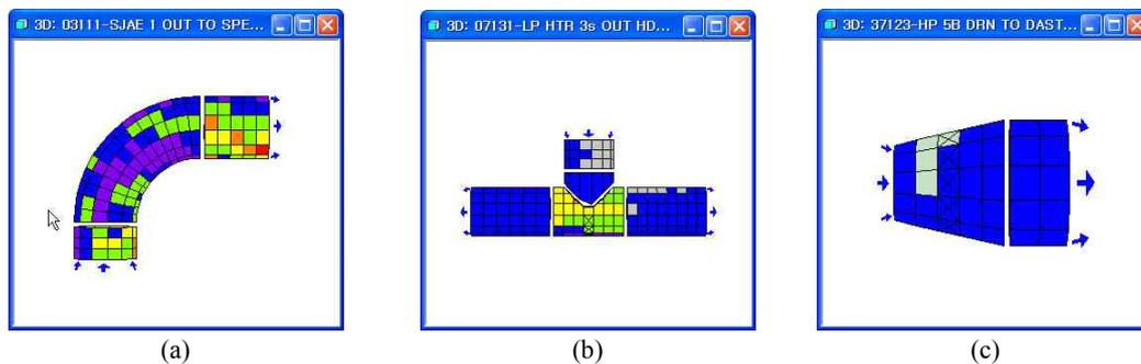
**Fig. 6.** Full and extended grid layout for fittings; (a) Elbow (b) Tee (c) Reducer or Expander.
