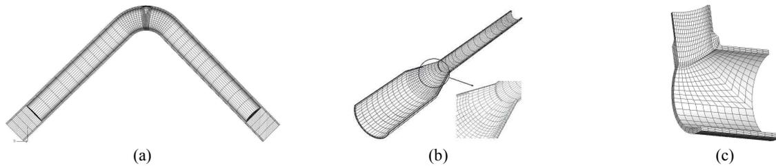
Fig. 12. Examples of finite element analysis model for thinned pipe components : (a) elbow (b) reducer (c) tee.
