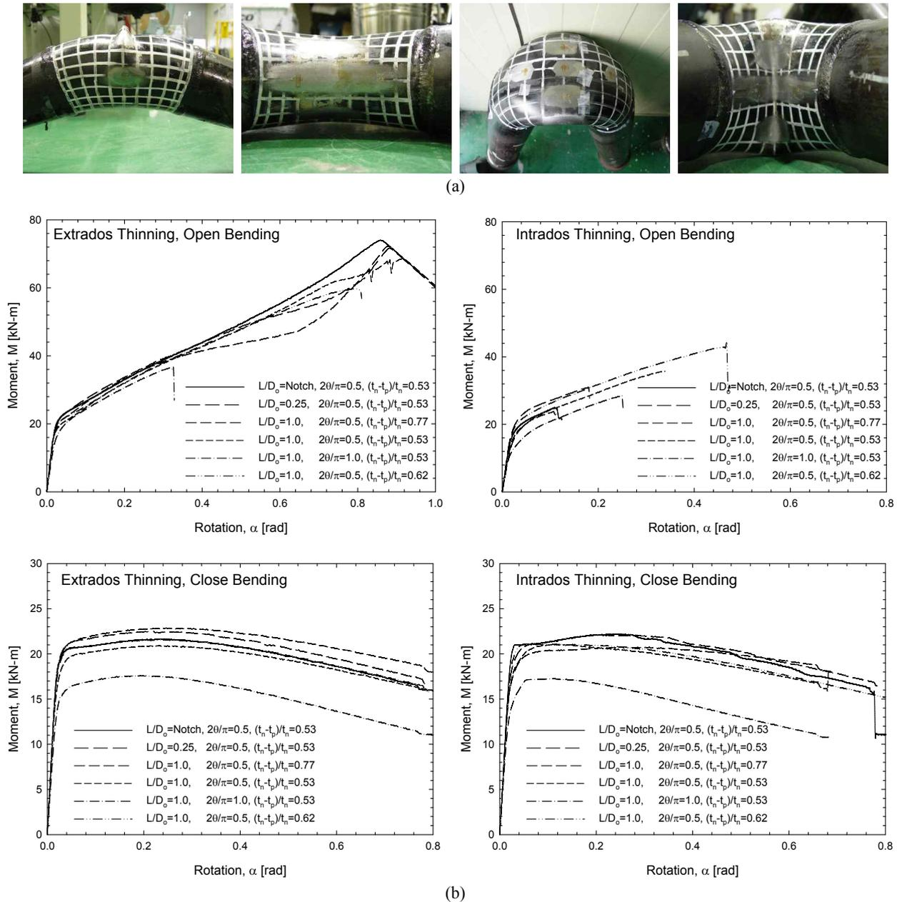
**Fig. 11.** Results of combined load tests of wall-thinned elbows : (a) failure modes according to the thinning location and the bending direction (b) moment behaviours according to the thinning location and the bending direction.
