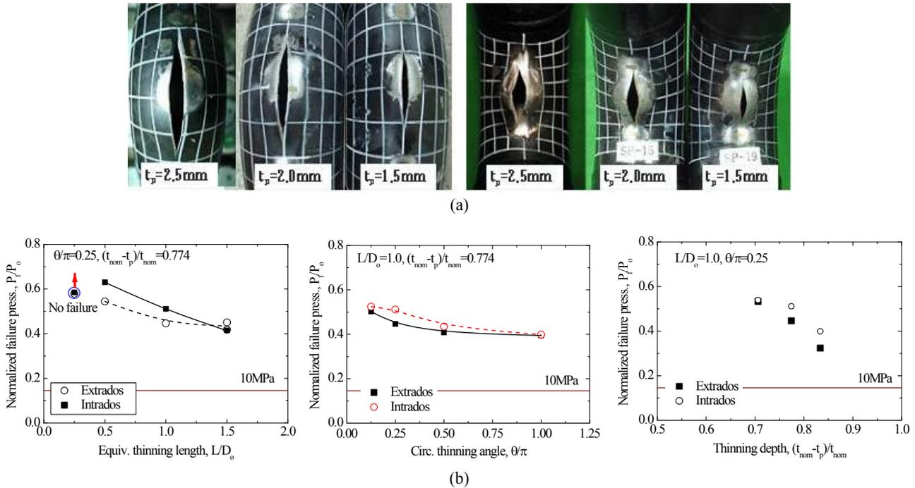
**Fig. 10.** Results of burst tests of wall thinned elbows : (a) burst modes according to the thinning location and the minimum thickness (b) comparison of burst pressure according to the thinning dimension.
