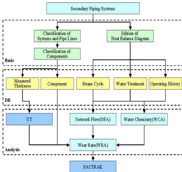
Fig. 4. Utilization of CHECWORKS™ program in TPMP.
