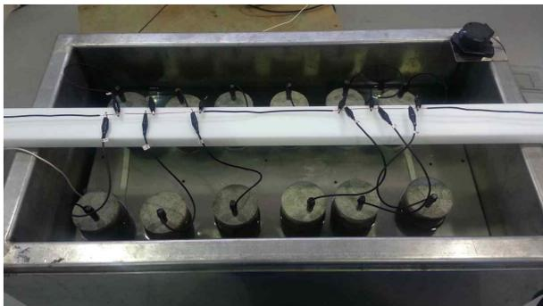
**Fig. 2.** Electrochemical accelerating corrosion test.
