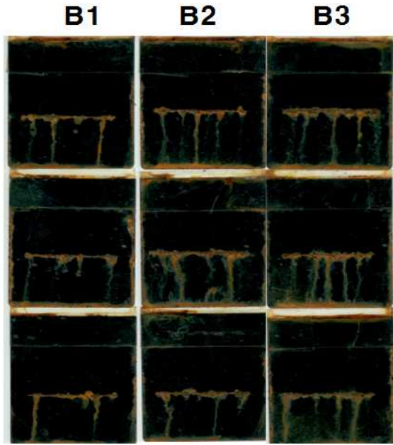
Fig. 5. Cyclic Corrosion Test results of the samples.
