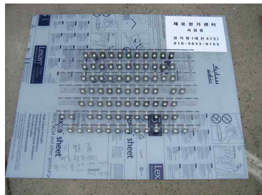
Fig. 4. Corrosion standard specimens set in outdoor.
