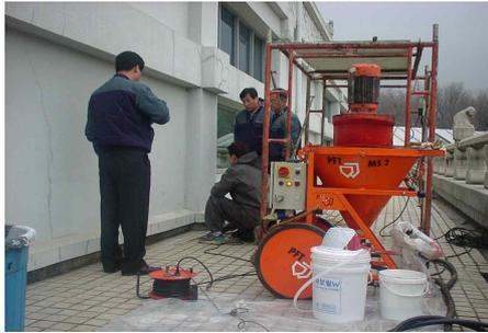
Fig. 12. Sealant injection equipment.
