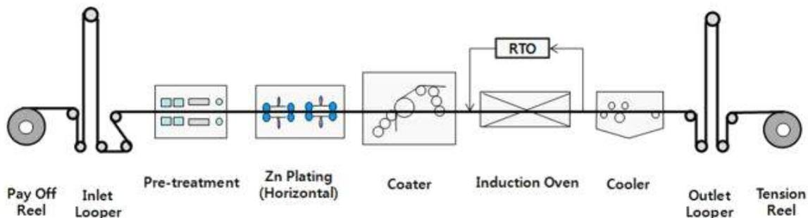
Fig. 1. In-line EGL layout for production of black resin coated steel sheet.
