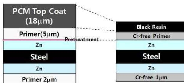
Fig. 4. Thinner coated layer of new product compared to conventional PCM steels.
