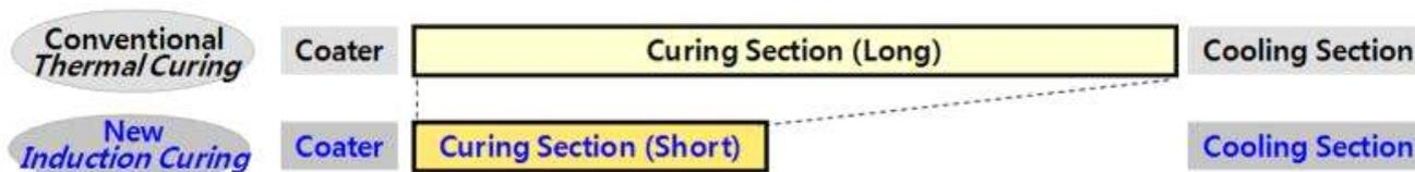
Fig. 3. Process differentiation between conventional thermal curing oven for PCM steels and induction curing oven for new product.
