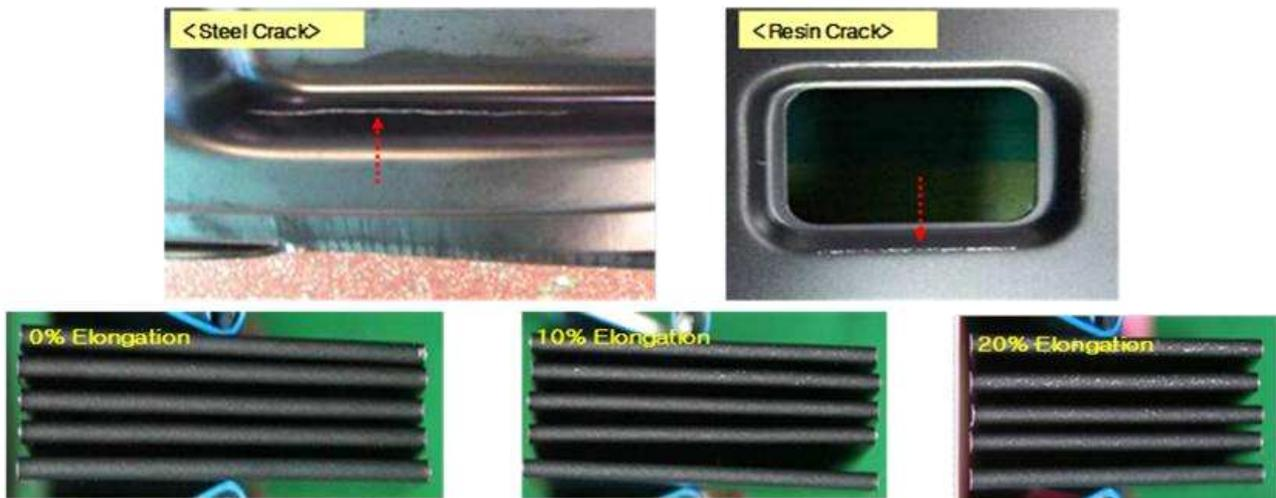
Fig. 6. During the press forming, both steel crack and resin crack occurred due to poor press formability of the layer (Top). Enhanced formability evaluation by OT bending evaluation after 0%, 10% and 20% elongation of new product (Bottom).
