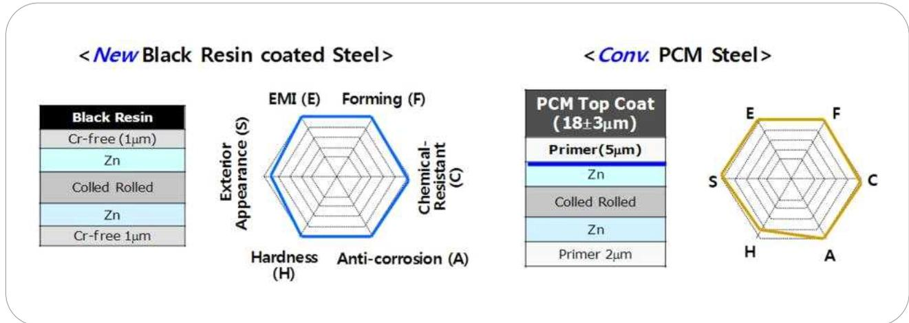
Fig. 7. Comparison in quality performances between new product and conventional PCM steel.
