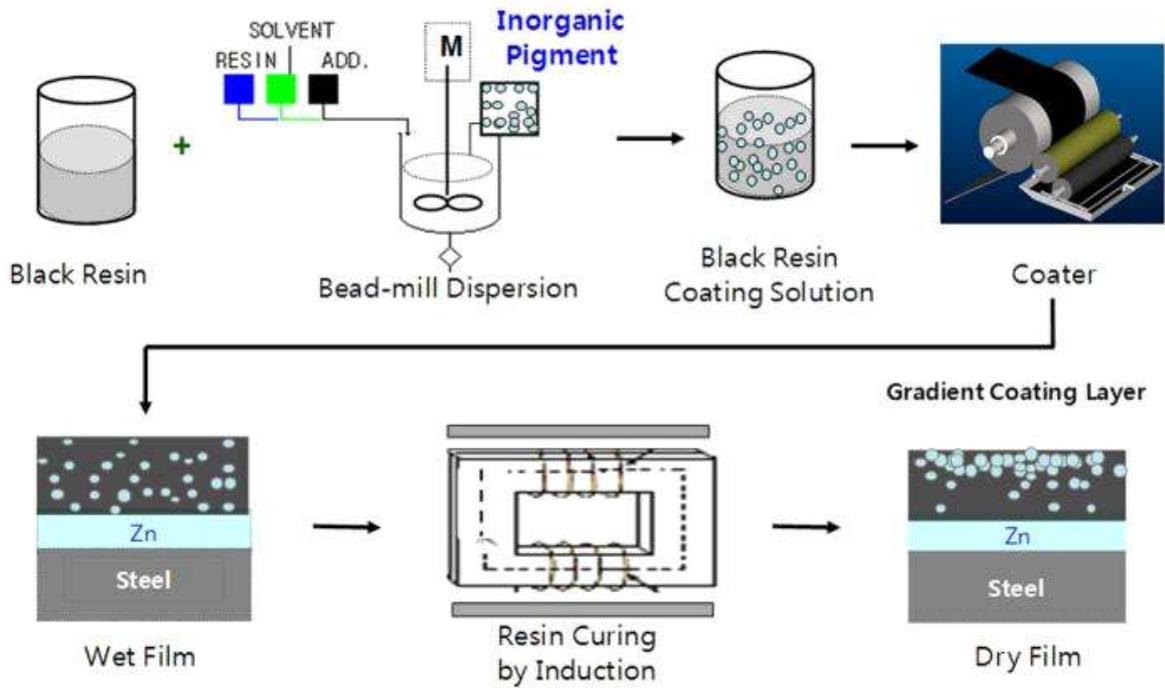
Fig. 5. Preparation of composite solution and formation of gradient coating layer during induction curing.
