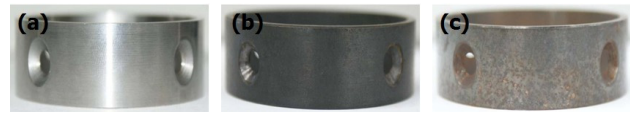
Fig. 9. Specimen appearance (a) after polishing, (b) tested in DO < 1 ppb and then cleaning with ultrasonic, (c) tested in DO = 1.5 ppm and then cleaning with ultrasonic.
