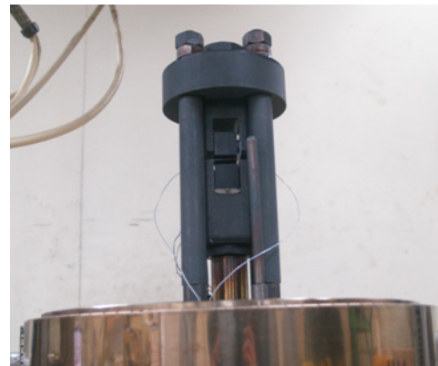
Fig. 3. Assembly of specimen after insulating.
