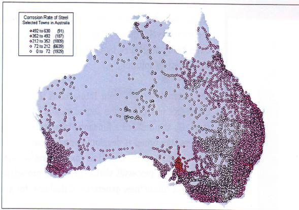
Corrosion rate of steel in selected towns in Australia
