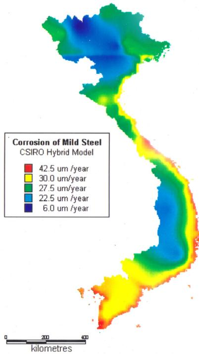
Fig. 4. Corrosion map of Viet nam by IDW Model.
