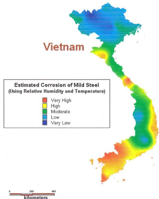
Fig. 3. Corrosion map of Vietnam by Holistic Model.
