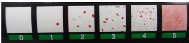
Fig. 9. Information summary to convert number values on chart to total acid producing bacteria counts of the soils.
