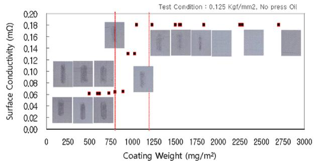
Fig. 6. Typical correlation between the coating weights vs. electrical conductivity, corrosion resistance, and abrasion property on the organic polymer-based resin coated steels.
