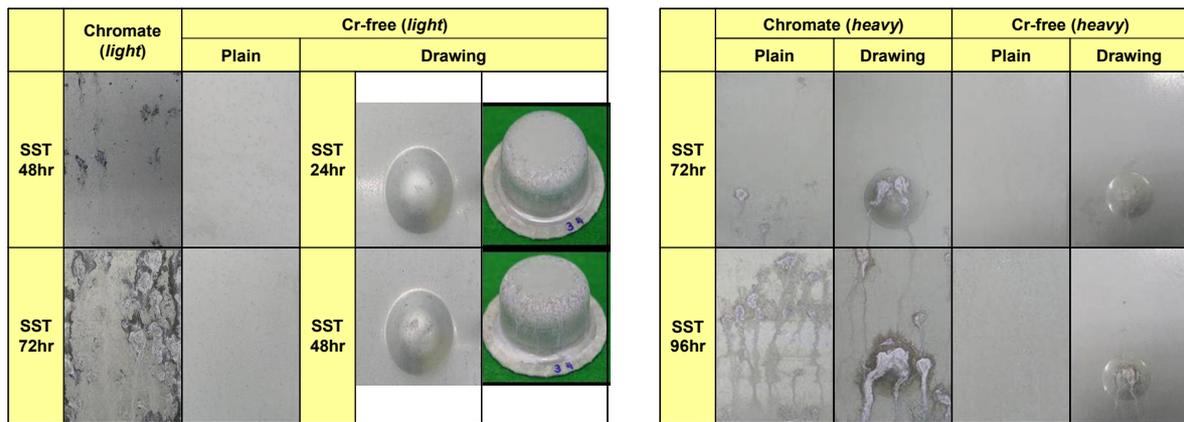
Fig. 2. Corrosion resistance for the chromate and Cr-free coated steels with light (*left*) and heavy (*right*) coating weights.
