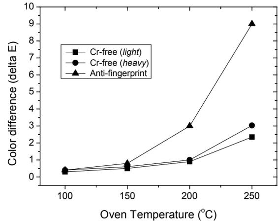
Fig. 5. Thermal tolerance tests for the Cr-free (*light & heavy*) and polymer-based anti-fingerprint coated steels.
