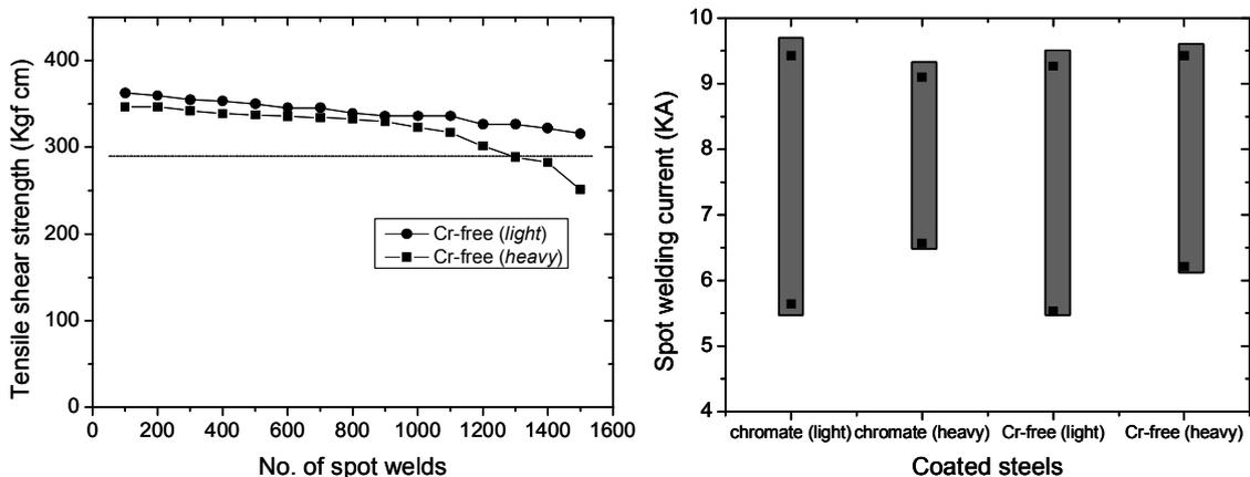
Fig. 3. Continuous spot welding performance of the Cr-free coated steels (*left*) and spot welding currents (*right*).
