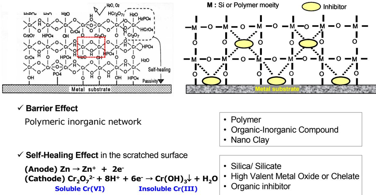
Fig. 1. Concept of Cr-free development in the coating layer. Chromate (*left*) and Cr-free (*right*) coating layer.
