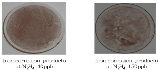
Fig. 7. Filtered iron corrosion products of condensate system during test.
