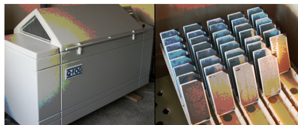
Fig. 2. Prohesion test equipment.
