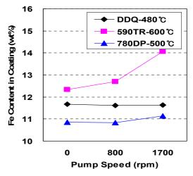
Fig. 8. Comparison of galvannealing rate with snout pump speed and steel types.
