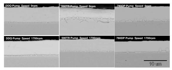
Fig. 6. Structure of galvanized coating layer with and without snout pumping.
