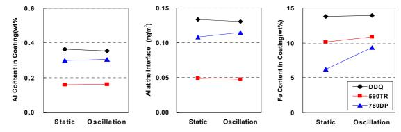
Fig. 1. Comparison of coating composition for the galvanized and galvannealed samples.
