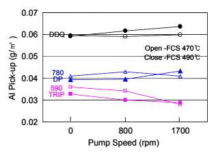
Fig. 5. Variation of Al pick-up at the interface with snout pump speed and strip entry temperature.
