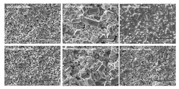
Fig. 3. Surface structure of the galvannealed coating for static and oscillating experiments.
