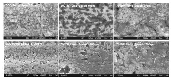
Fig. 7. Surface structure of interfacial layer for hot-dip galvanizing with and without snout pumping.
