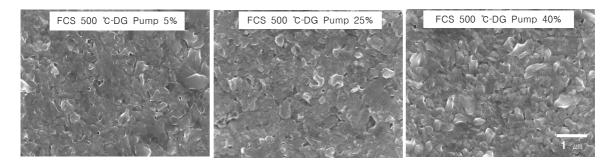
Fig. 9. Surface structure of inhibition layer with zinc pump ratio and FCS temperature (No.A coil)
