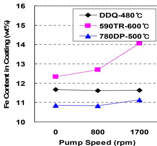
Fig. 8. Comparison of galvannealing rate with snout pump speed and steel types.
