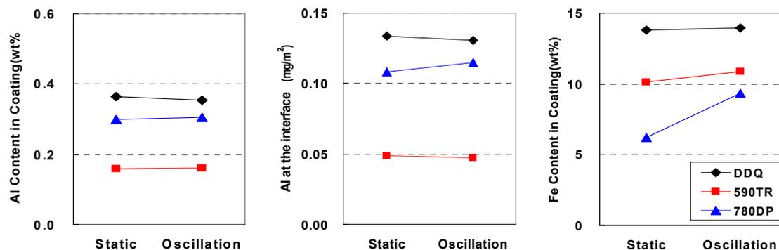
Fig. 1. Comparison of coating composition for the galvanized and galvannealed samples.
