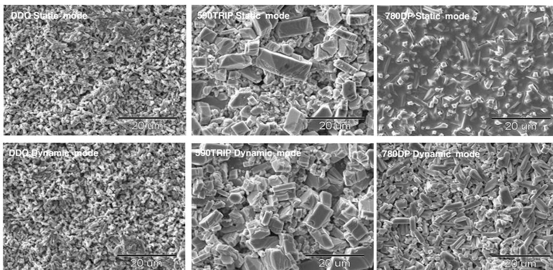
Fig. 3. Surface structure of the galvanized coating for static and oscillating experiments.
