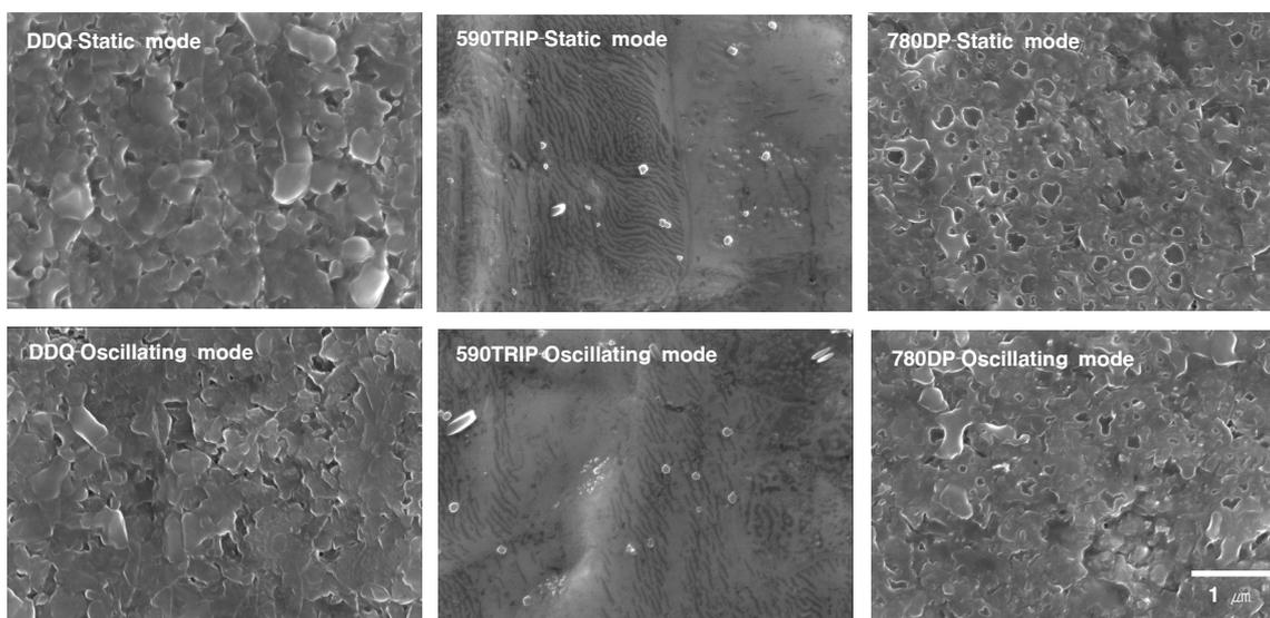
Fig. 2. Surface structure of interfacial layer for hot-dip galvanizing for static and dynamic experiments.
