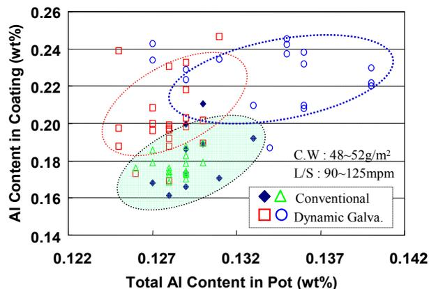
Fig. 11. Relations of Al content in zinc bath with Al content in coating layer.
