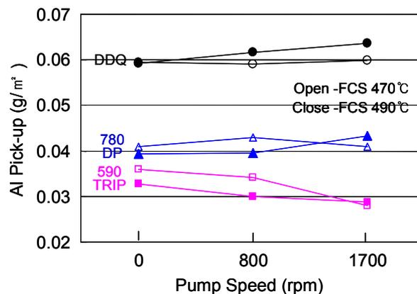
**Fig. 5.** Variation of Al pick-up at the interface with snout pump speed and strip entry temperature.
