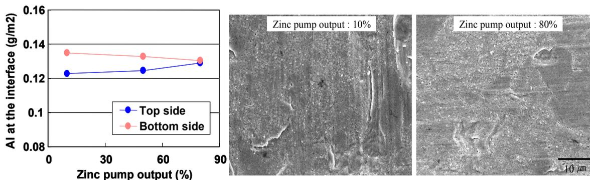
Fig. 10. Al pick-up at the interface and surface structure of interface layer with zinc pump ratio (No.B coil).
