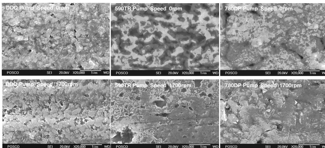
Fig. 7. Surface structure of interfacial layer for hot-dip galvanizing with and without snout pumping.
