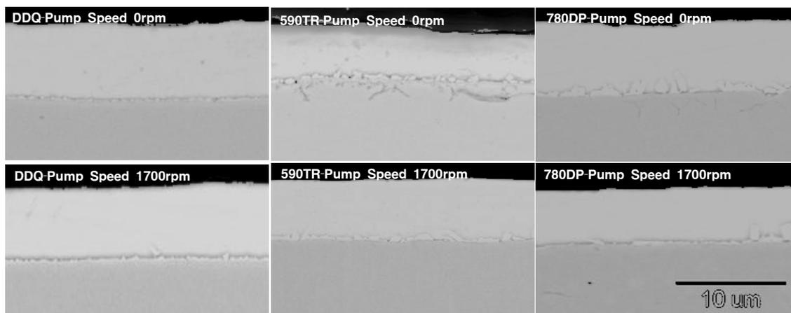
**Fig. 6.** Structure of galvanized coating layer with and without snout pumping.
