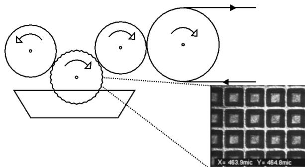
Fig. 2. Schematic of patterned roll coating and the surface image of an engraved roll.
