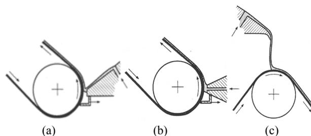
Fig. 3. Schematics of touchless coating methods. (a) slide coating; (b) slot coating; (c) curtain coating.
