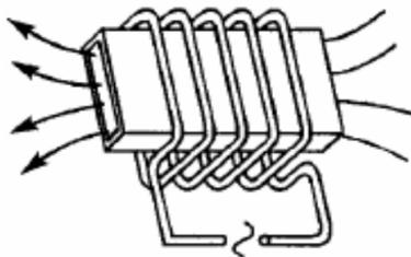
Fig. 4. Concept of strip induction heating.
