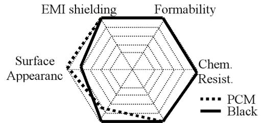
Fig. 6. Performance comparison between PCM and black resin coated steel.
