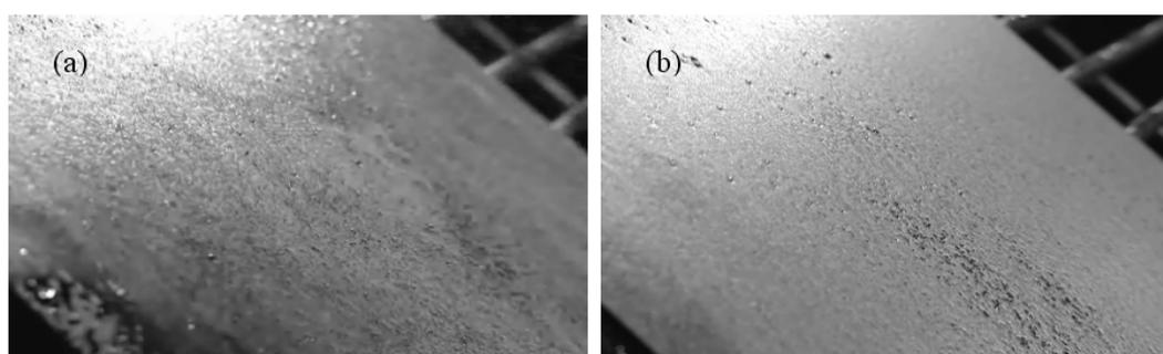
Fig. 8. Comparison of dirty steel surface after spraying water. Self cleaning surface (a) becomes much cleaner than conventional PCM surface (a).
