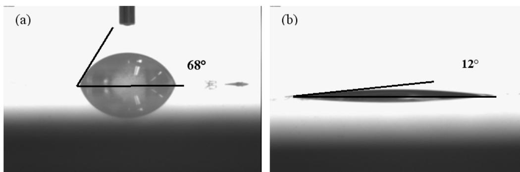
Fig. 7. Contact angle difference of water drop on the surface of conventional PCM (a) and self cleaning surface (b).
