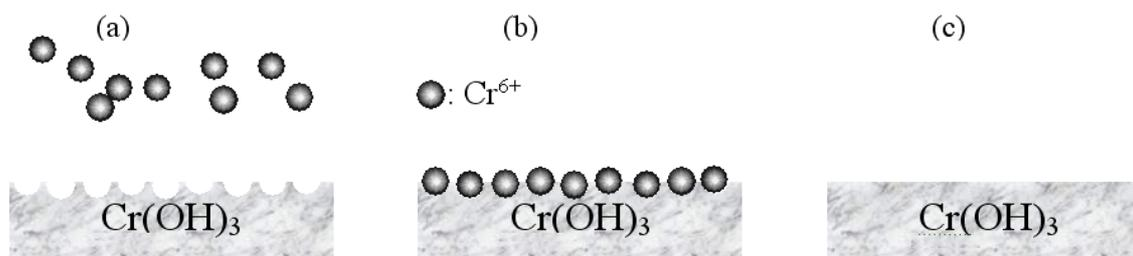
**Fig. 5.** Illustration of self healing effect by chromate coating. (a) mobile  $\text{Cr}^{6+}$  ions move around chromate layer; (b)  $\text{Cr}^{6+}$  ions adheres to the defect surface of chromate layer; (c) surface defects are healed.
