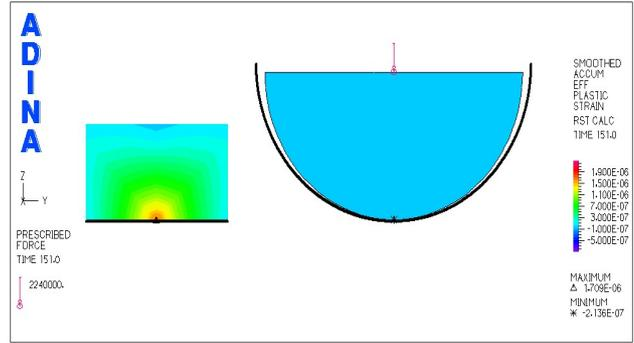
**Fig. 1a.** Accumulated plastic strain in the sleeve and shaft of an industry bearing with a radial clearance of 10 mm.
