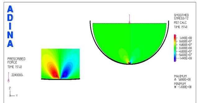
**Fig. 1b.** Shear stress  $\sigma_{yz}$  in the sleeve and shaft of an industry bearing with a radial clearance of 10 mm.
