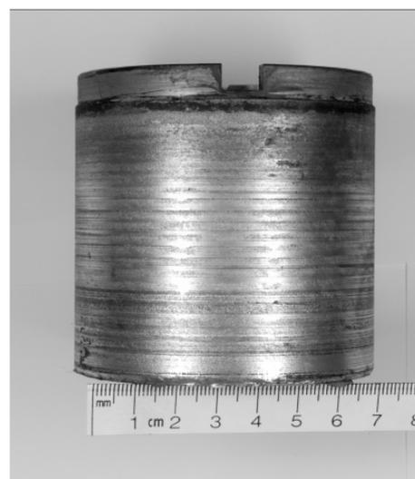
**Fig. 2.** The surface smoothness of the SiAlON blocks and the WC-coated 316L SS sleeve has been noticeably improved following a laboratory test, owing to the grinding/polishing effect induced by the sliding contact in the test.
