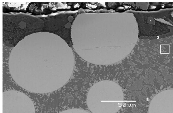
**Fig. 3.** Cross-section of a WC-coated 316L SS sleeve after being tested against a SiAlON bushing in a GL bath. The binder of the coating corroded severely, and its support of the WC particles was weakened. A transverse crack developed within the carbide slightly ahead of the advancing corrosion front in the coating. The particle (1) and the intermetallic layer forming at the corrosion front (2) are both of the  $\tau_5$  composition.
