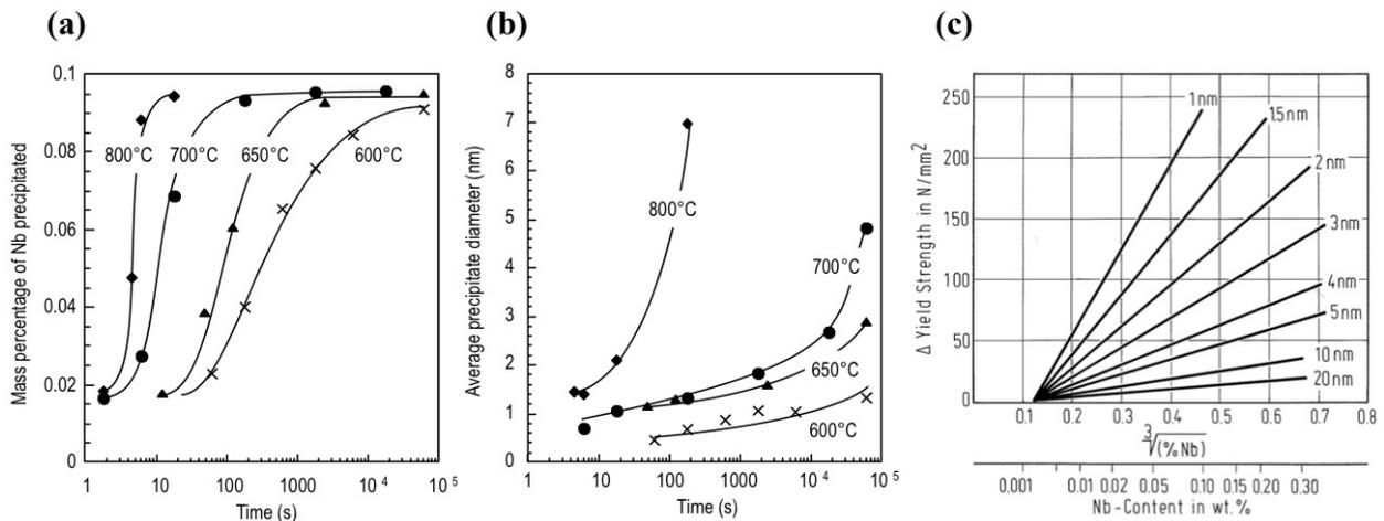
**Fig. 4.** Precipitation behavior of hot rolled strip with 0.03%C-1.7%Mn-0.1%Nb after low temperature coiling; (a) Fraction of precipitated solute Nb after annealing treatment at various temperatures and times; (b) Coarsening behavior of NbC precipitate depending on annealing temperature and duration; (c) Influence of NbC precipitate amount and average size on yield strength increase.
