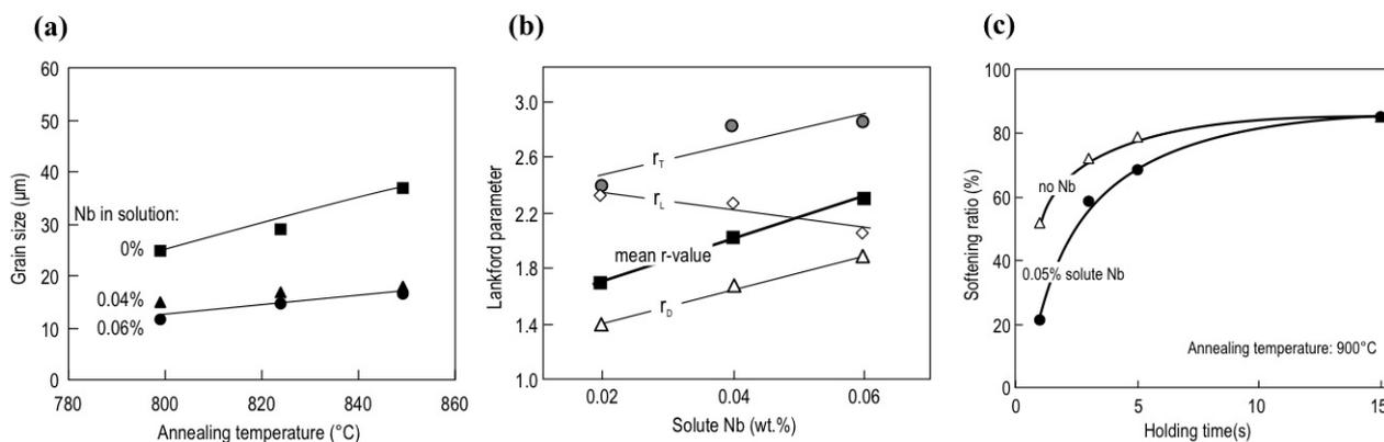
**Fig. 5.** Effects of adding Nb to a Ti-stabilized IF high strength steel (0.003%C-0.002%N-0.07%Ti-Mn-P); (a) Evolution of final grain size in function of annealing temperature at various solute Nb levels; (b) Evolution of r-value in function of the solute Nb level; (c) Softening behavior for annealing close to the  $A_{r1}$  temperature.
