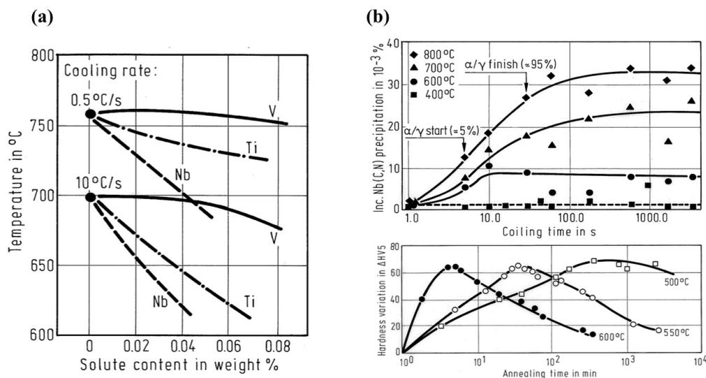
**Fig. 3.** (a) Dependency of  $A_{F3}$  temperatures on solute microalloying content in 0.1%C-1.5%Mn steel with standard austenite grain size of 100  $\mu\text{m}$ ; (b) Effect of isothermal holding on Nb precipitation in 0.04%C-0.5%Mn-0.04%Nb steel.
