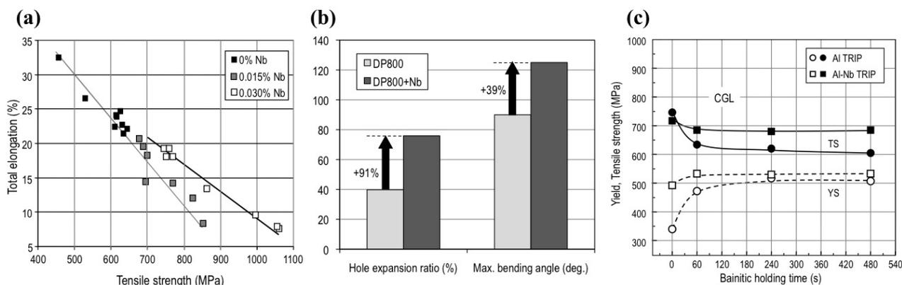
**Fig. 6.** (a) Effect of Nb addition on property balance in low-carbon DP800 steel (0.08%C-2.0%Mn-0.5%Cr); (b) Effect of Nb induced grain refinement on hole expansion and bending behavior in DP800 steel; (c) Property balance in TRIP steel (0.2%C-1.5%Mn-2.0%Al-0.045%Nb) in function of bainitic holding.
