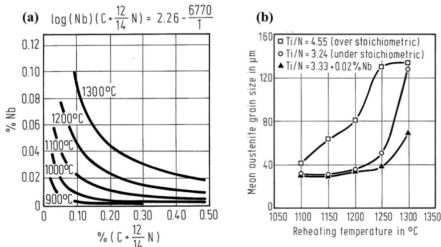
**Fig. 2.** (a) Solubility isotherms of Nb as a function of C and N in austenite; (b) Effect of non-dissolved particles on the austenite grain size during slab reheating.
