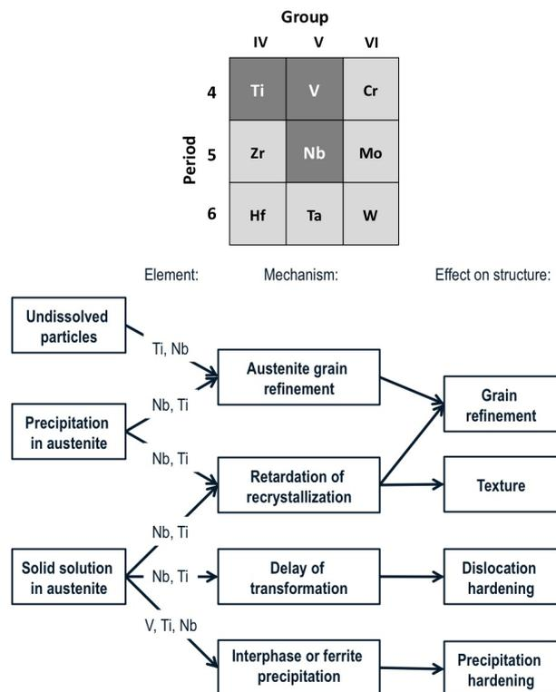
**Fig. 1.** Transition metals for special alloying purposes and metallurgical effects of microalloying elements (Nb, Ti, V).
