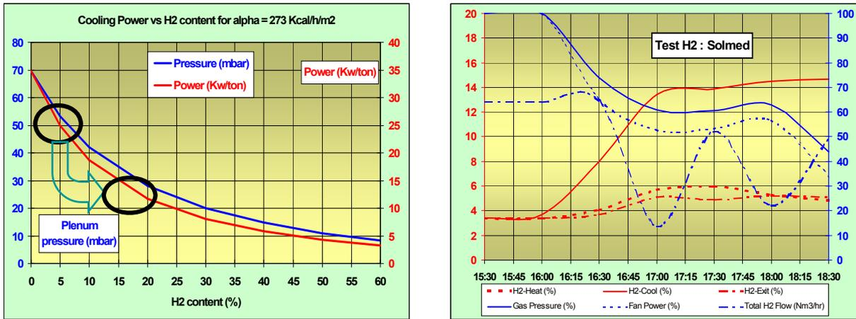
Fig. 2. (left) Effect of hydrogen content on plenum pressure and fan power
