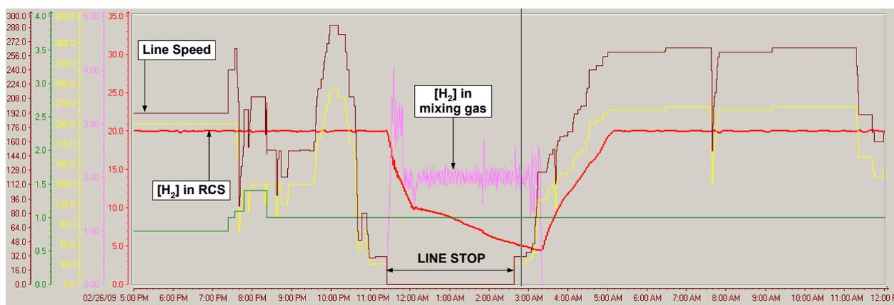
**Fig. 4.** Rapid cooling hydrogen concentration versus line speed in CAL N°1. Line stop induces the return to the use of classical HN<sub>x</sub> mixing gas
