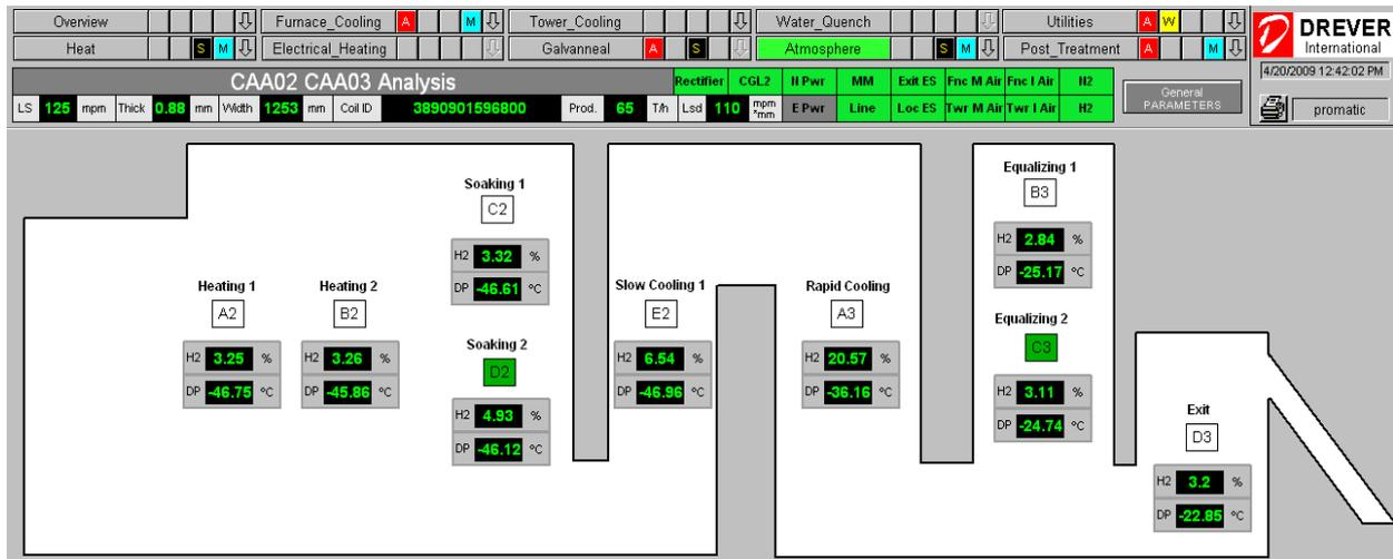
Fig. 6. Rapid cooling high hydrogen confinement in Shougang ShunYi CGL N°1
