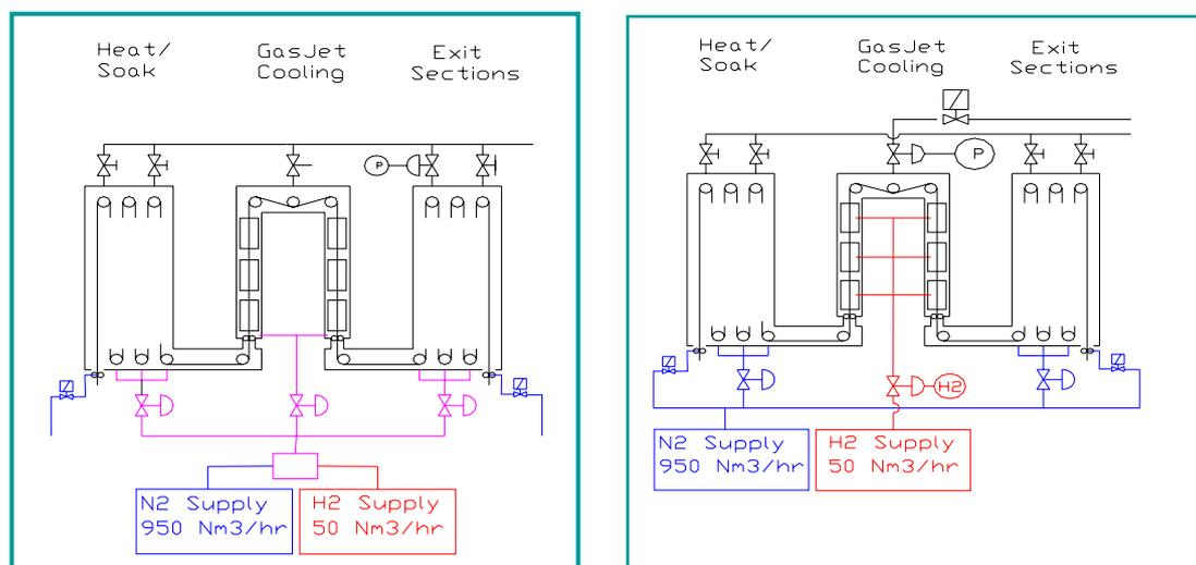
**Fig. 1.** (left) Classical injection of HN<sub>x</sub> mixture in the furnace
