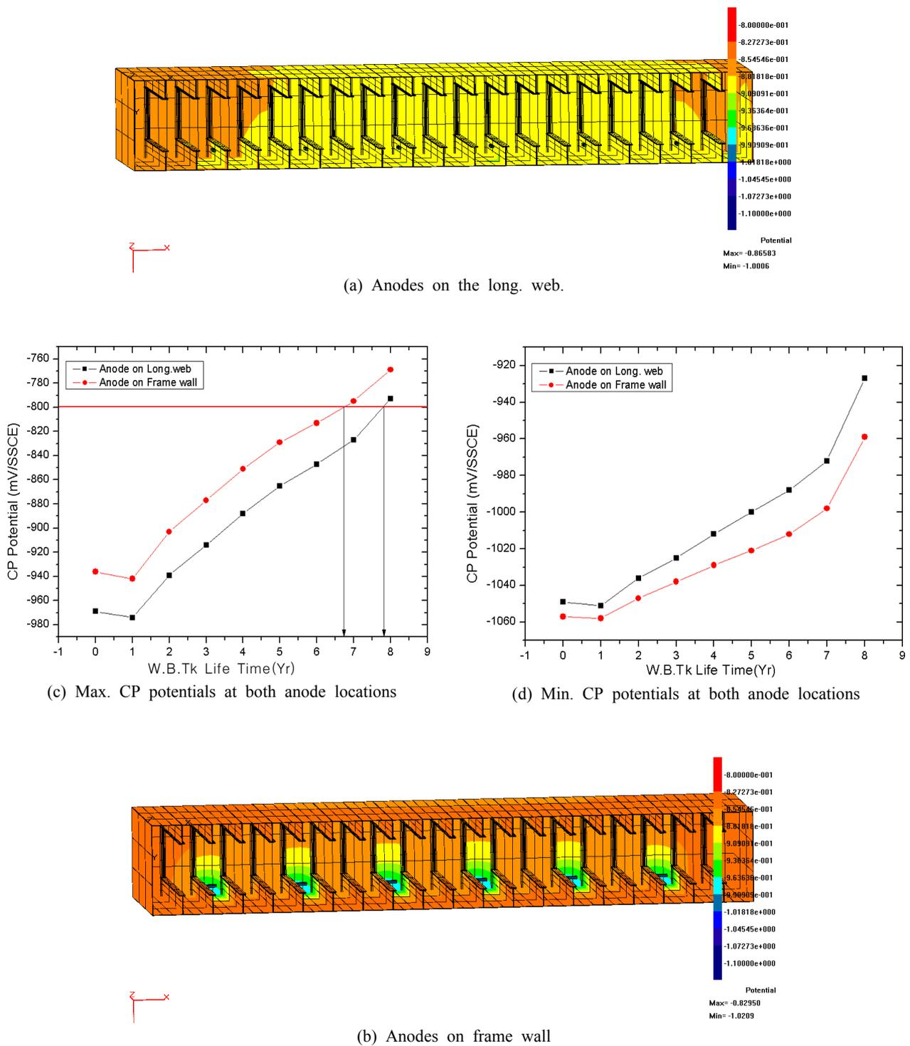
Fig. 8. CP potential results of Bottom W.B. Tank
