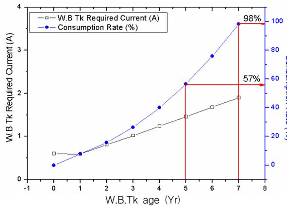
(a) Anode consumption rate with over time
