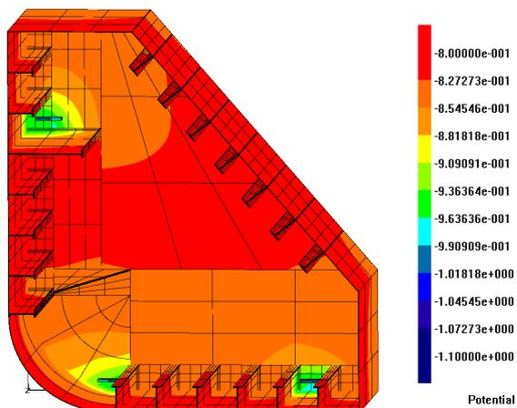
(b) Anodes on frame wall
