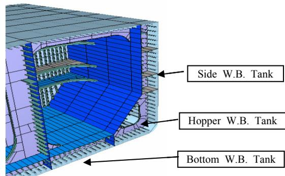
Fig. 2. Typical water ballast tanks of a crude oil tanker.
