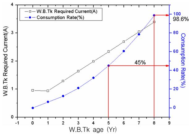
(a) Anode consumption rate with over time
