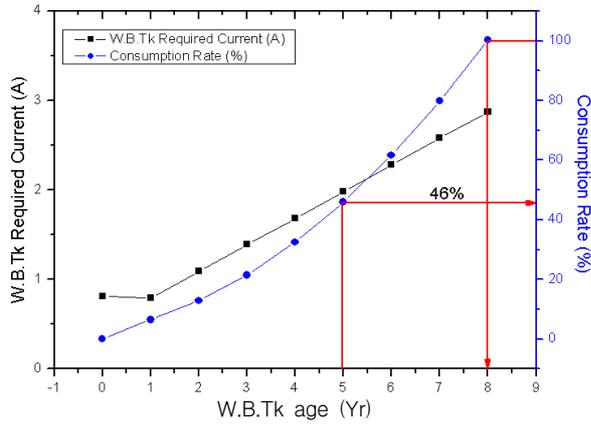
(a) Anode consumption rate with over time
