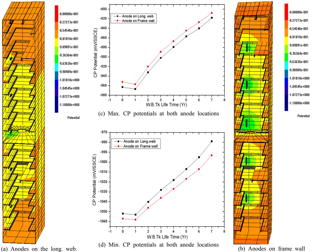
Fig. 6. CP potential results of Side W.B. Tank
