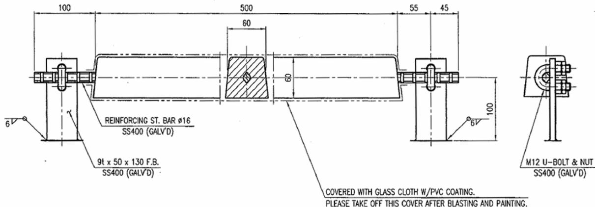
Fig. 1. The dimensions of selected Al-anode.
