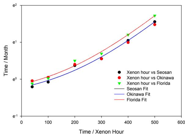
**Fig. 4.** The correlation between outdoor exposure and accelerated samples' gloss changes
