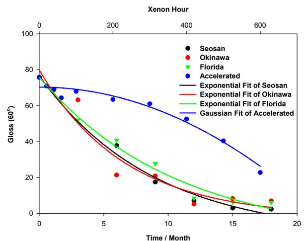
**Fig. 3.** Gloss changes at different outdoor exposure sites and accelerated samples.
