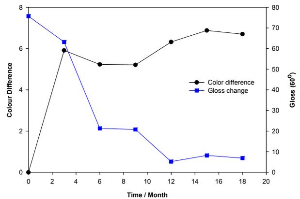
**Fig. 1.** Color and gloss changes as a function of time for outdoor exposed samples
