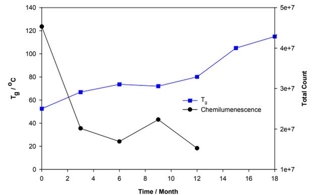
**Fig. 2.** Glass transition temperature and chemiluminescence spectroscopic changes as a function of time for outdoor exposed samples
