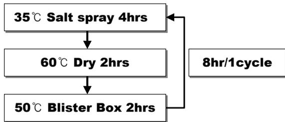
**Fig. 1.** The condition of cyclic corrosion test.
