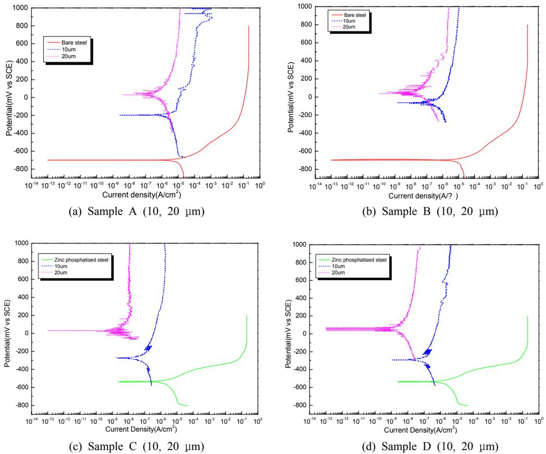
Fig. 4. The results of potentiodynamic polarization with variable film thickness
