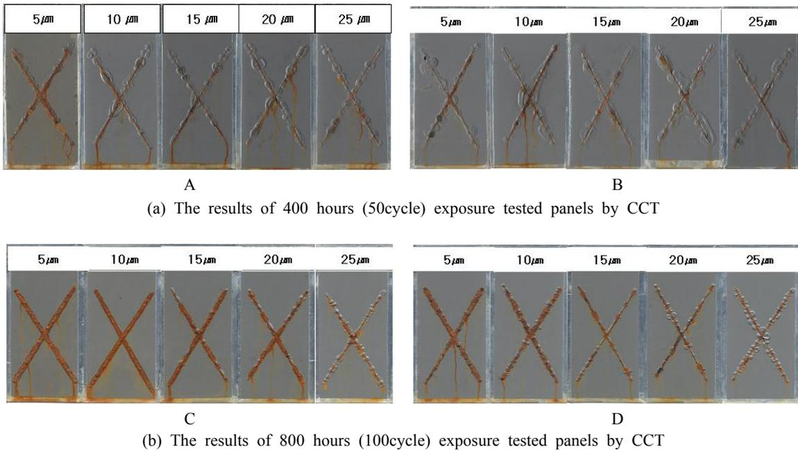
Fig. 3. The results of CCT exposure tested panels (thickness: 5, 10, 15, 20, 25  $\mu\text{m}$ )
