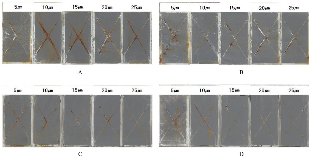
**Fig. 2.** The results of 1200 hours exposure tested panels by SST (thickness: 5, 10, 15, 20, 25  $\mu\text{m}$ )
