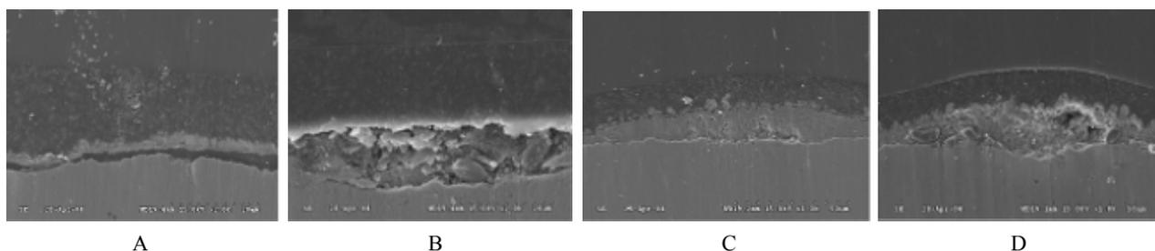
**Fig. 5.** The cross-sectional SEM images of different primer after 21days immersion at 50 $^{\circ}\text{C}$  with EIS performed.
