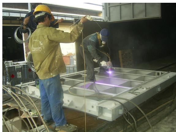
**Fig. 2.** Some images of zinc spray application to water intake gates for Mekong water basin Sand blast (left) and Zinc spray (right)
