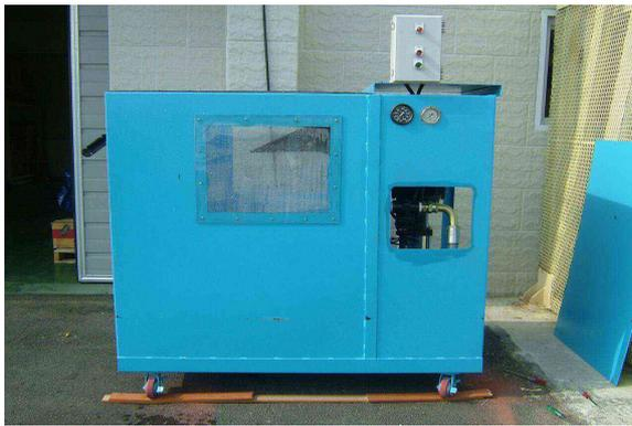
Fig. 4. Water-jet cavitation erosion tester
