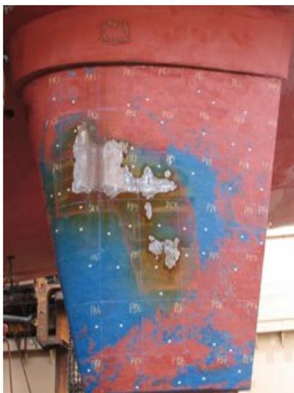
Fig. 2. Typical cavitation induced corrosion damage of ship's rudder<sup>1)</sup>
