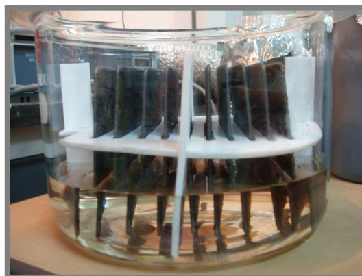
Fig. 5. Immersion test in sulfuric acid of fluoroelastomers(95% H<sub>2</sub>SO<sub>4</sub>, 90°C)
