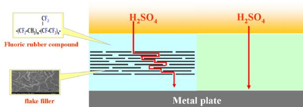
Fig. 4. Corrosion prevention mechanism of flake filler
