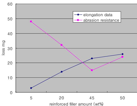
Fig. 7. Characteristics related to elasticity of coating with various amount of reinforced filler
