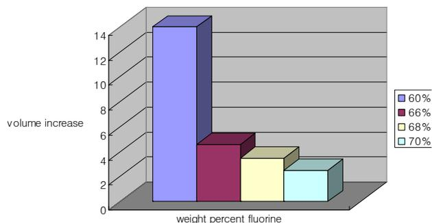
Fig. 3. Weight percent fluorine and acid resistance comparison
