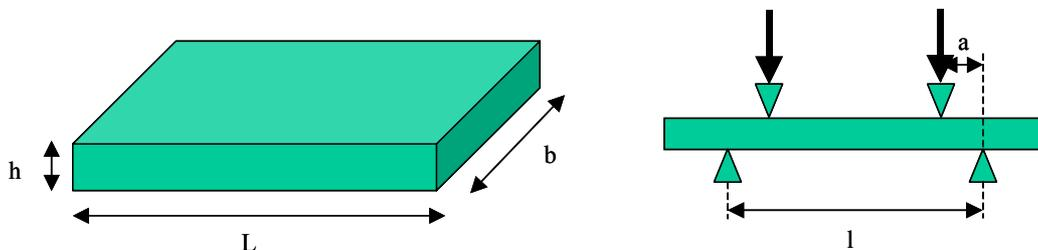
**Fig. 2.** Definition of the parameters used for the calculation of stress and sag for the four point bending tests
