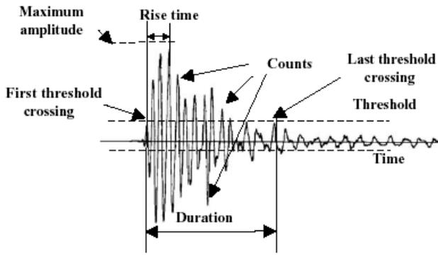
Fig. 3. Definition of the main shape parameters of an acoustic signal, from<sup>4)</sup>
