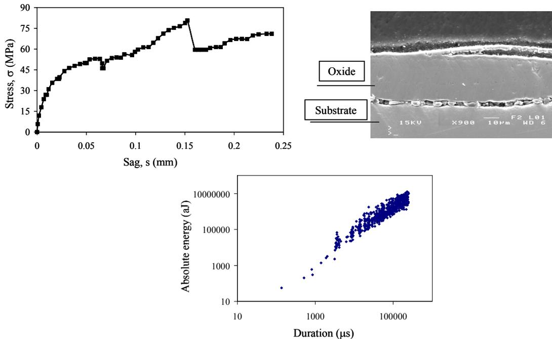
**Fig. 8.** Stress-Sag curve, acoustic emission diagram and SEM view of a cross-section of the steel oxidized at 900°C under a dry N<sub>2</sub>, and sollicitated at T=700°C
