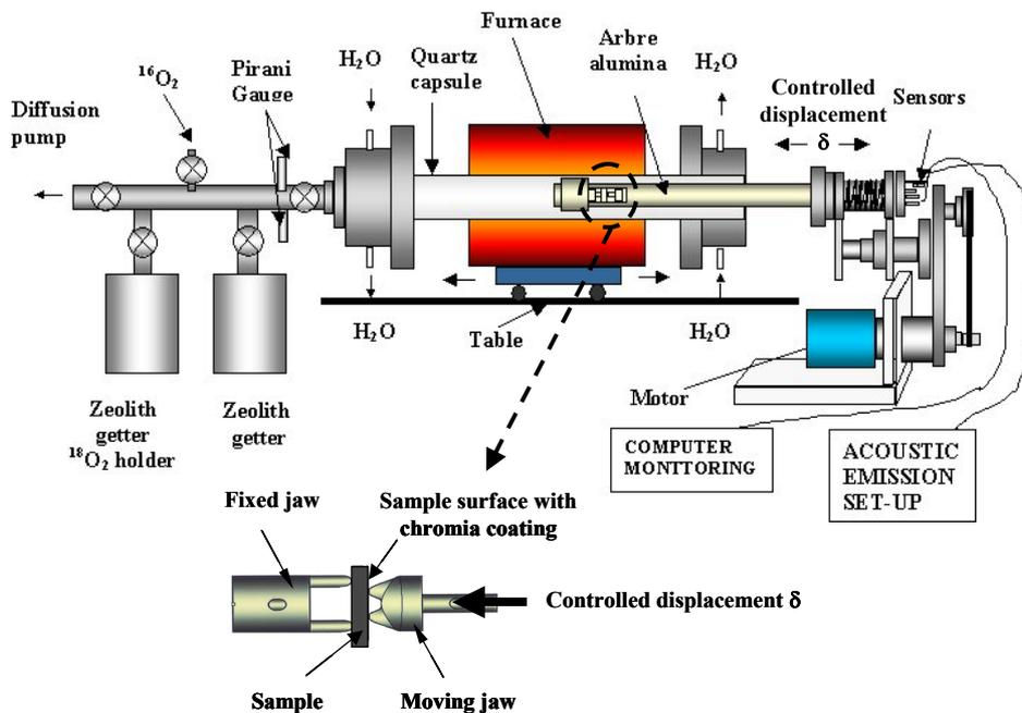
Fig. 1. Schematic drawing of the high temperature four point bending test under controlled atmosphere
