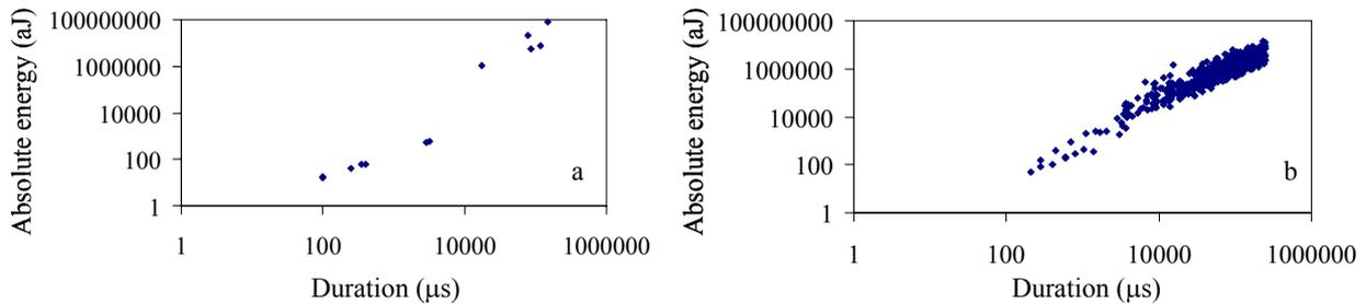
Fig. 6. Acoustic emission diagrams (absolute energies of the acoustic events versus their duration) for the steel oxidized under the N<sub>2</sub>+H<sub>2</sub>O mixture at 900°C, and sollicited (a) at 900°C and (b) at 700°C
