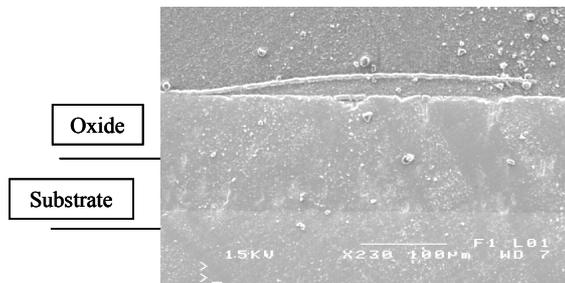
Fig. 5. Stress-Sag curve and SEM view of a cross-section of the steel oxidized at 900°C under a N<sub>2</sub>+H<sub>2</sub>O mixture, and sollicited at T=900°C
