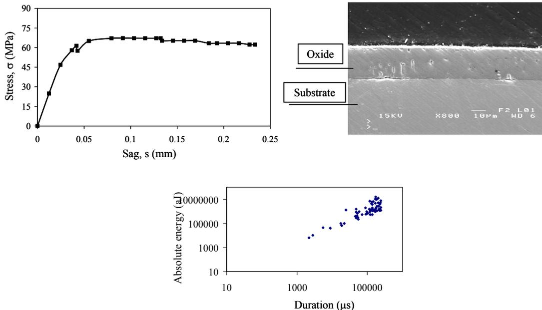
Fig. 7. Stress-Sag curve, acoustic emission diagram and SEM view of a cross-section of the steel oxidized at 900°C under a dry N<sub>2</sub>, and sollicited at T=900°C
