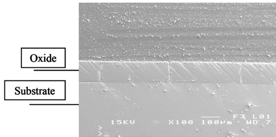
Fig. 4. Stress-Sag curve and SEM view of a cross-section of the steel oxidized at 900°C under a N<sub>2</sub>+H<sub>2</sub>O mixture, and sollicited at T=700°C
