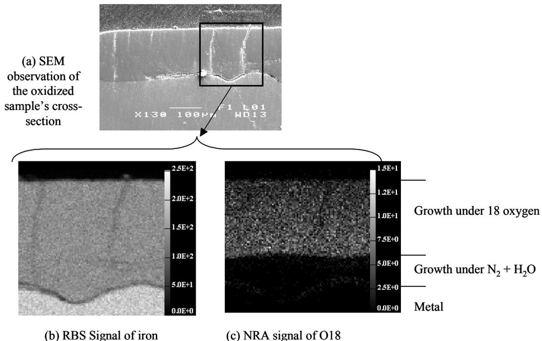
Fig. 9. SEM cross-section observation and corresponding chemical analysis by a nuclear microprobe of a sample annealed 9 minutes under N<sub>2</sub>+H<sub>2</sub>O at 900°C, sollicitated at 900°C and annealed 2h under <sup>18</sup>O<sub>2</sub> at 900°C
