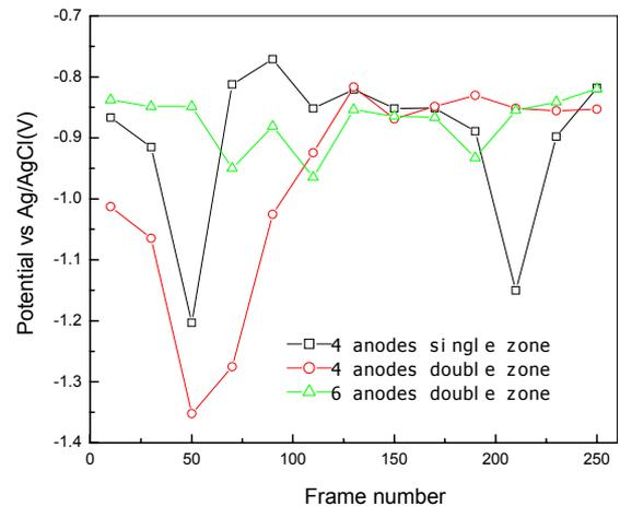
Fig. 5. Comparisons of single zone and double zone ICCP system of model ship
