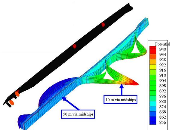
Fig. 4. Ship underwater steady electric field signature prediction(at a depth of 5 m from waterline)
