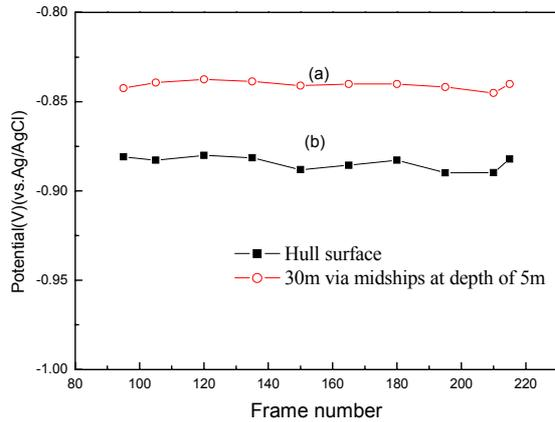
Fig. 6. Ship underwater steady electric field signature of model ship (Six anodes double zone ICCP system)
