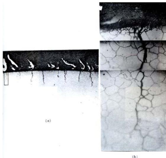
**Fig. 1.** Transgranular SCC observed in an operating nuclear power plant.
