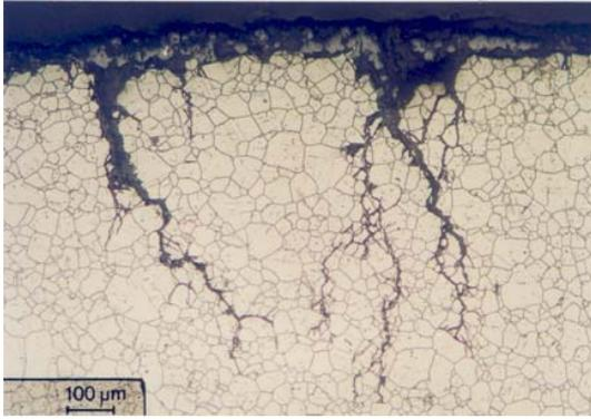
**Fig. 4.** TGSCC observed in alloy 690 TT tested in 40 % NaOH with 5000 ppm of lead at 315°C for 21 days.
