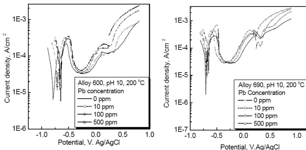
Fig. 7. Effect of the lead contents on the anodic polarization of alloy 600 and 690 at 200 °C.<sup>10)</sup>
