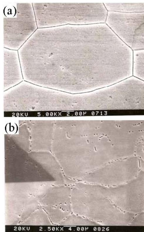
Fig. 2. Grain boundary microstructures etched in phosphoric acid: (a) alloy 600 MA and (b) 600 TT.
