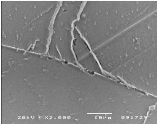
**Fig. 5.** Transition of crack path from IG into TG in the alloy 690 TT tested in 40 % NaOH solution with 5000 ppm lead at 315°C.
