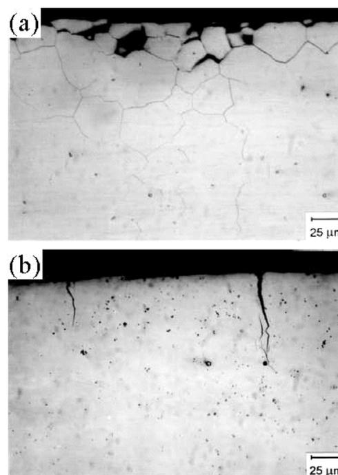
Fig. 3. Different cracking modes in 10 % NaOH test solution with 100 ppm lead at 315°C: (a) intergranular in alloy 600 MA and (b) transgranular in alloy 600 TT.
