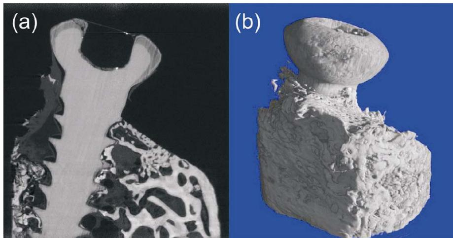
**Fig. 4.** Synchrotron-radiation microtomography (SRμCT) images showing the 3D orientation of the magnesium screw inside the sheep bone. Left image (a) shows a longitudinal section through the 3D reconstructed and stacked data-sets of a AZ31 magnesium screw that was implanted into sheep bone for 3 months. Right image (b) shows the external appearance of the same data-set as displayed in the left image (a).
