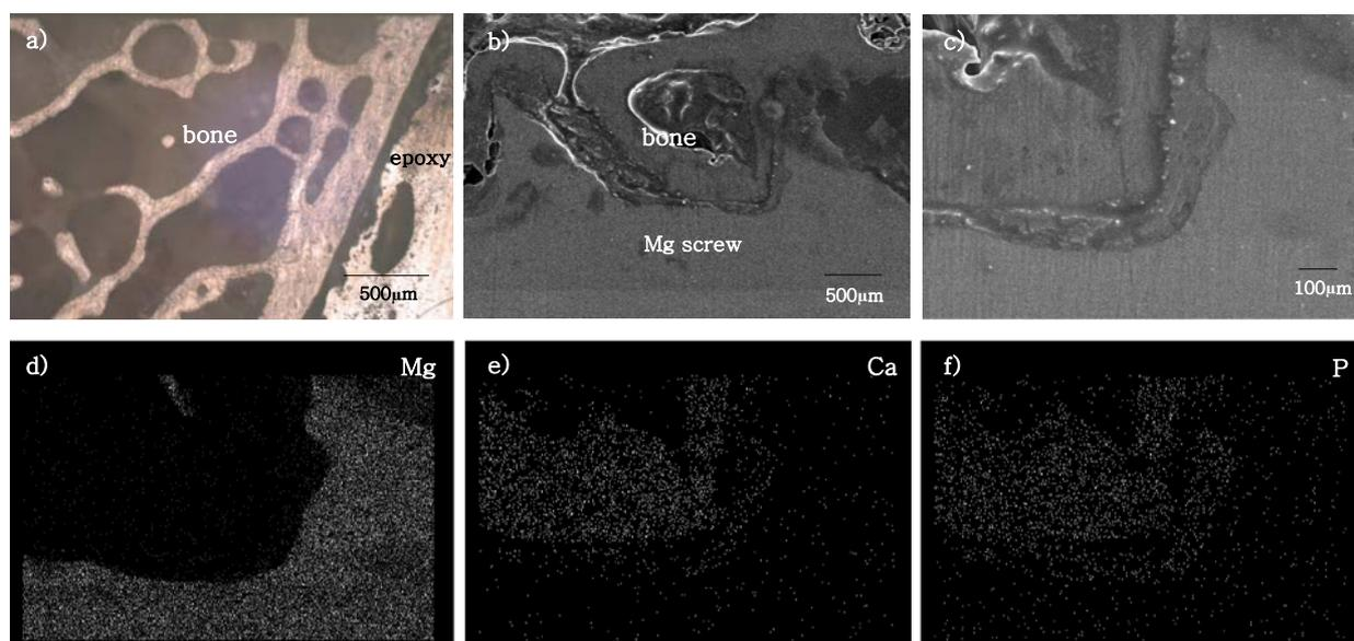
**Fig. 5.** (a) Optical microscope image of the bone mounted in epoxy, and scanning electron microscope images of magnesium alloy AZ31 screw implant-bone interface, (b) at low magnification, (c) at high magnification; and elemental mapping analyses of the interface showing elements: (d) magnesium, (e) calcium, and (f) phosphorus.
