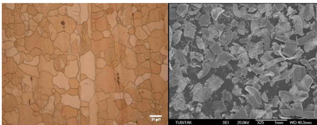
**Fig. 1.** Optical micrograph showing the microstructure of the magnesium alloy AZ31 bone screw, and the particulate magnesium material employed in this study.
