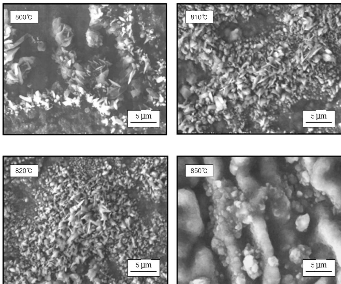
**Fig. 1.** External surface of the  $\text{Al}_2\text{O}_3$  scale formed on a steel FeCrAl during 24 h oxidation in  $\text{SO}_2+0,01\%$   $\text{O}_2$  gas mixture at temperatures 800, 820, 830 and  $850^\circ\text{C}$ , respectively.
