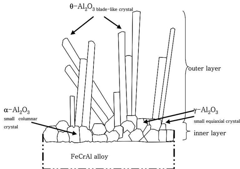
**Fig. 7.** Scheme of scale structure formed on the FeCrAl steel oxidized 24 h under  $SO_2+1\% O_2$  atmosphere at  $820^\circ C$ .
