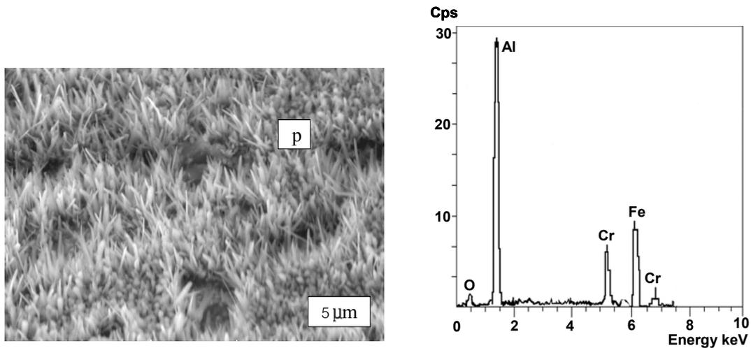
**Fig. 2.** External surface of the  $Al_2O_3$  scale formed on FeCrAl steel oxidized 24 h in  $SO_2+1\% O_2$  atmosphere at  $820^\circ C$  and EDX analysis at point P.
