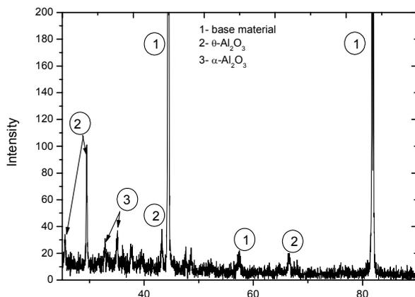
**Fig. 3.** Diffraction patterns of the  $Al_2O_3$  scale formed on a FeCrAl steel oxidized 24 h in  $SO_2+1\% O_2$  atmosphere at  $820^\circ C$ .
