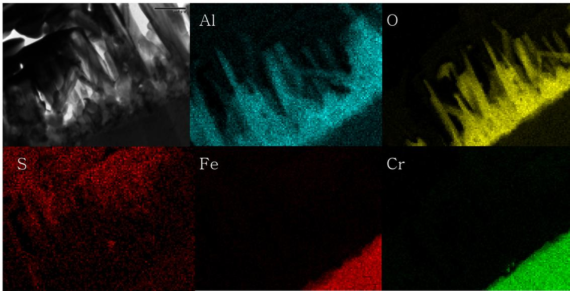
**Fig. 4.** Chemical microanalysis from TEM image of the  $\text{Al}_2\text{O}_3$  scale formed on the FeCrAl steel oxidized 24 h in  $\text{SO}_2+1\% \text{O}_2$  atmosphere at  $820^\circ\text{C}$ .
