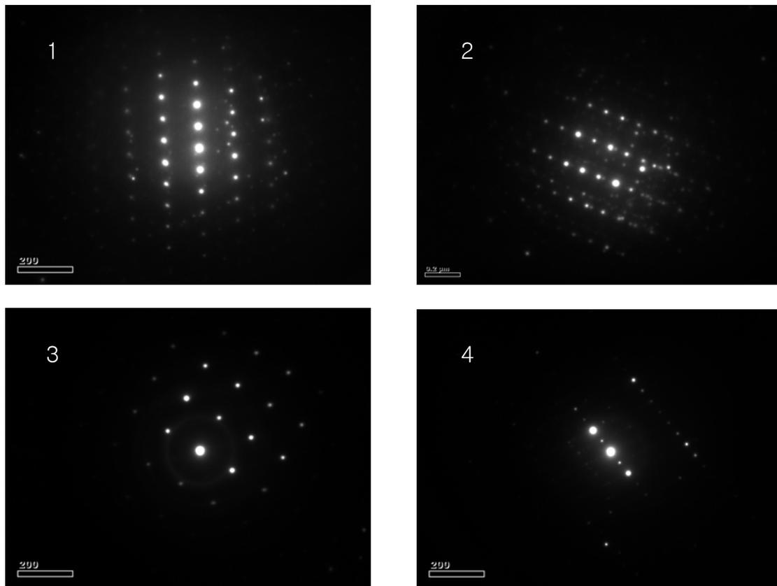
**Fig. 6.** Diffraction patterns of the  $Al_2O_3$  scale formed on the FeCrAl steel oxidized 24 h under  $SO_2+1\% O_2$  atmosphere at  $820^\circ C$ : point (1) small equiaxial grain from inner oxide layer corresponds to  $\gamma-Al_2O_3$ , (2) small columnar grain from inner oxide layer corresponds to  $\alpha-Al_2O_3$ , (3) blade-like crystal and (4) the next neighbour crystal are  $\theta-Al_2O_3$ .
