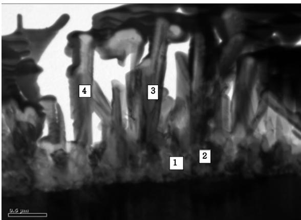
**Fig. 5.** TEM image of the  $\text{Al}_2\text{O}_3$  scale formed on the FeCrAl steel oxidized 24 h under  $\text{SO}_2+1\% \text{O}_2$  atmosphere at  $820^\circ\text{C}$ .
