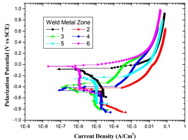
Fig. 6. Polarization curves of WM in case of various electrodes in sea water solution.
