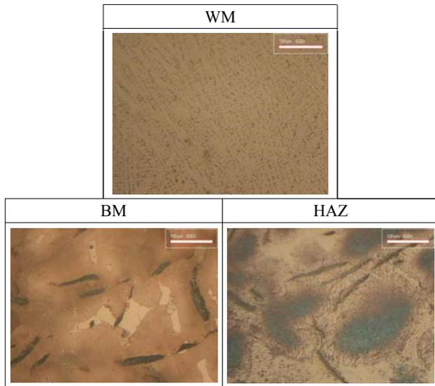
Fig. 8. Optical microstructures of HAZ, BM and WM ( $\times 600$ )
