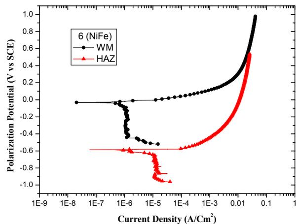
Fig. 7. Polarization curves of WM and HAZ in sea water solution.
