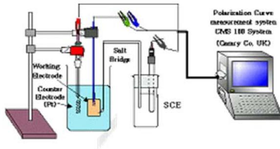
**Fig. 2.** Schematic diagram of experimental apparatus for polarization curves.
