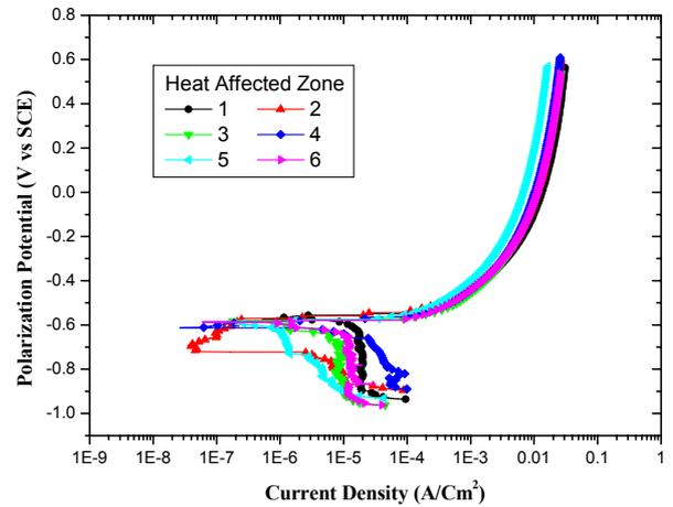
Fig. 5. Polarization curves of HAZ in sea water solution.
