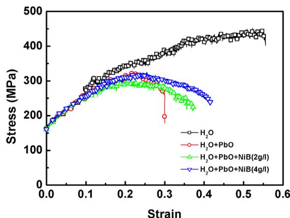
Fig. 2. Stress-strain curves of Alloy 600 HTMA obtained from the SSRT tests in pure water with/without additives.
