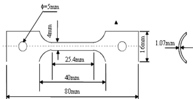
Fig. 1. Design of SSRT specimens.
