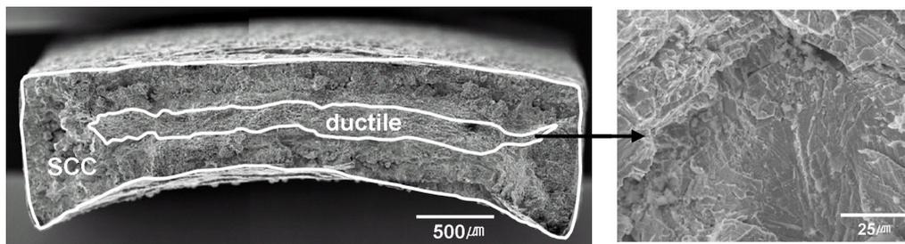
**Fig. 4.** SEM micrographs of the gauge surface of Alloy 600 HTMA strained in H<sub>2</sub>O+10,000ppm PbO.
