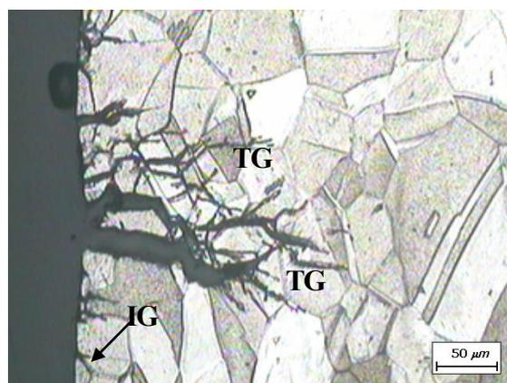
Fig. 6. Optical micrograph of SCC occurring in Alloy 600 HTMA strained in H<sub>2</sub>O+10,000ppm PbO.
