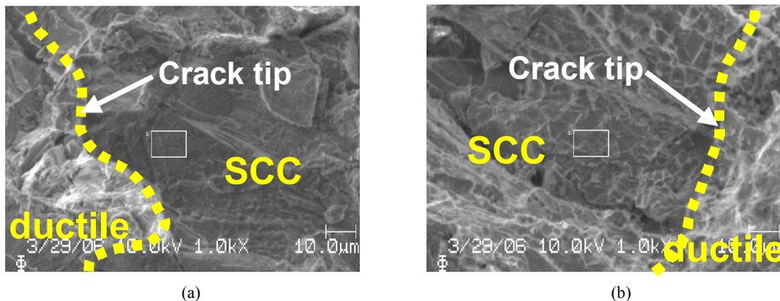
**Fig. 7.** Fracture surfaces showing the crack tips of Alloy 600 specimens tested in (a) H<sub>2</sub>O+PbO and H<sub>2</sub>O+PbO+NiB(4g/l) at 315°C. AES analysis done in the rectangular regions with white boundary on the fracture surfaces
