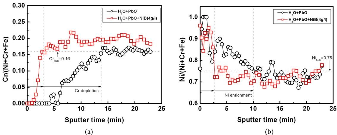
**Fig. 8.** Depth profile of oxide film compositions formed on the fracture surface at crack tip. Depth profiles of (a) Cr and (b) Ni.
