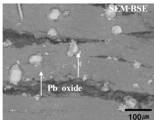
Fig. 5. SEM micrograph of the gauge surface of Alloy 600 HTMA strained in H<sub>2</sub>O+10,000ppm PbO.
