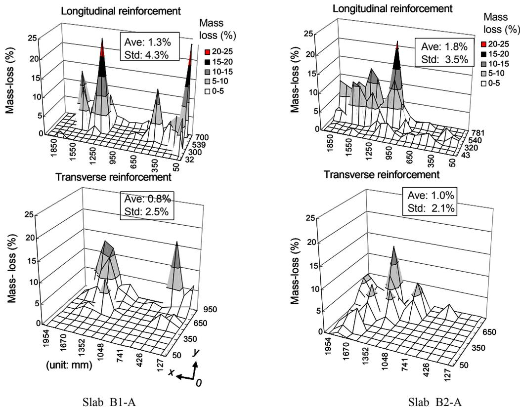
Fig. 5. Distribution of mass-loss of reinforcement
