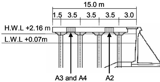
Fig. 1. Cross sectional view of open-pile structure in Port H
