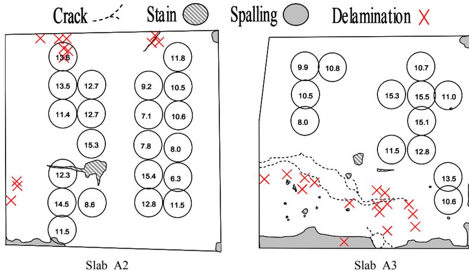
Fig. 3. Distribution of surface chloride ion concentration ( $\text{kg/m}^3$ )
