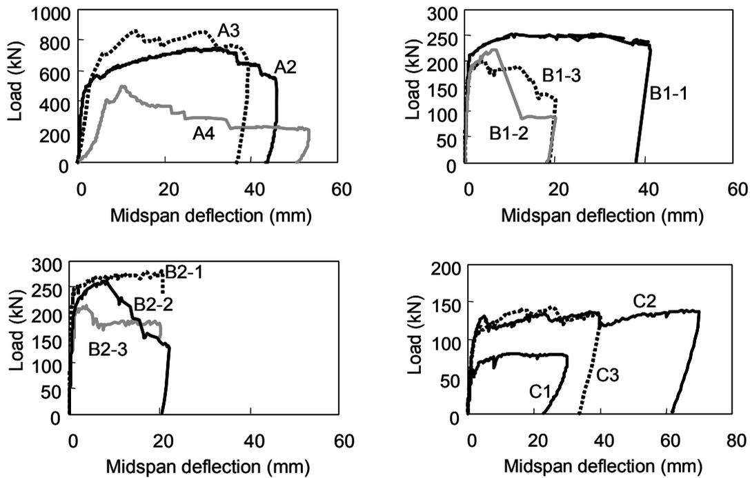
Fig. 8. Load-deflection curves of slabs
