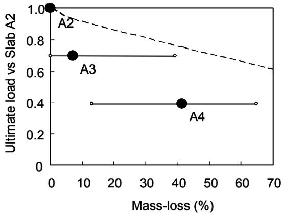
Fig. 9. Effect of variation of mass-loss on ultimate load
