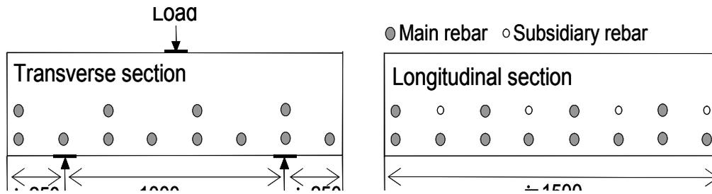
Fig. 2. Test setup and cross section of Slabs A2-A4
