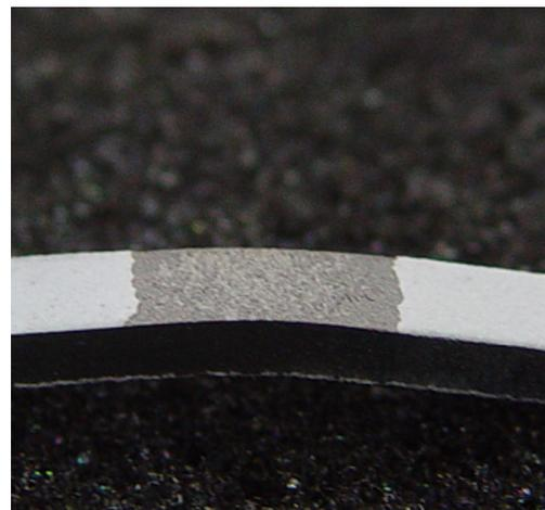
(b) HAp coating on titanium with heat treatment
