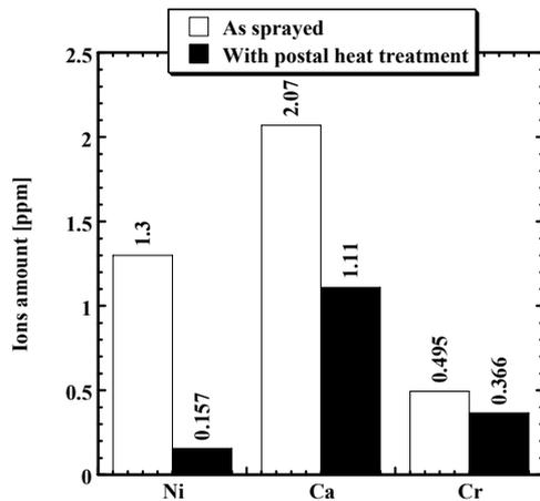
Fig. 2. Results of ICP analysis for plasma spray HAp/titanium coating on SUS316L in physiological saline.
