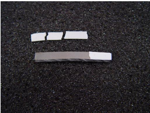
(b) HAp coating on titanium with heat treatment
