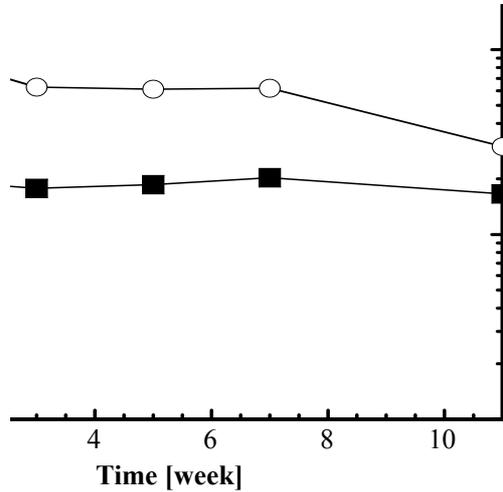
Fig. 1. Changes in corrosion resistance ( $R_c$ ) for HAp/titanium combined coatings in physiological saline at room temperature.
