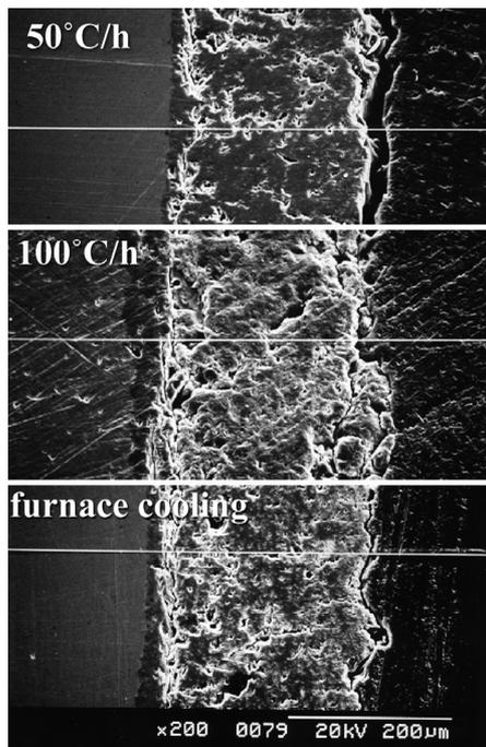
Fig. 5. Cross section profile of plasma spray HAp/titanium coating treated at different cooling rate.
