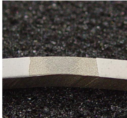
(a) HAp coating on titanium as sprayed
