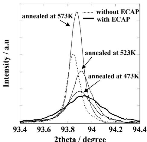
Fig. 9. Effect of annealing on the X-ray diffraction pattern of Al-Mg alloy processed by ECAP.
