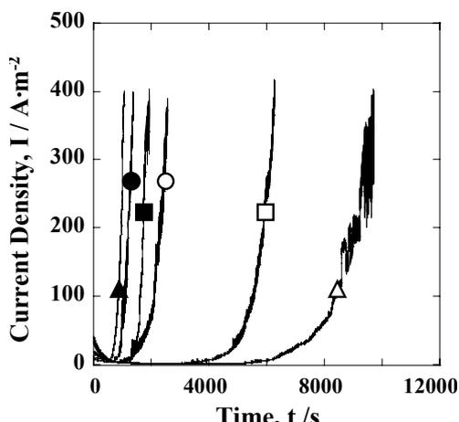
Fig. 4. Time-dependence of the anodic current density of Al-Mg alloy anodized at 100, 200 and 400 A·m<sup>-2</sup> while kept at constant potential of 1.2V in 0.2 mol·L<sup>-1</sup> of AlCl<sub>3</sub> solution. ○●: 100 A/m<sup>2</sup>, □■: 200 A/m<sup>2</sup>, △▲: 400 A/m<sup>2</sup>, ○□△: without ECAP, ●●■▲: with ECAP
