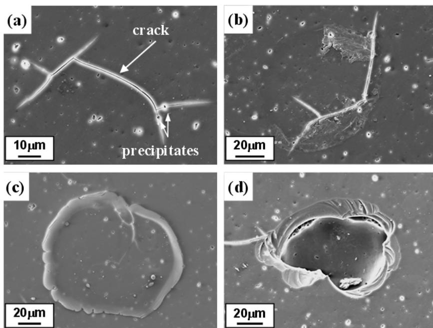
Fig. 6. SEM images of anodized Al-Mg alloy without ECAP after kept 1.2V in 0.2 mol·L<sup>-1</sup> of AlCl<sub>3</sub> solution.
