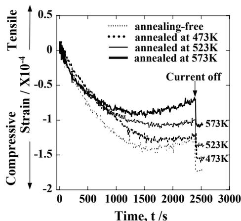
Fig. 8. Effect of annealing on the strain of Al-Mg substrates during anodization at 400 A·m<sup>-2</sup> in a solution containing 1.53 mol·L<sup>-1</sup> of H<sub>2</sub>SO<sub>4</sub> and 0.0185 mol·L<sup>-1</sup> of Al<sub>2</sub>(SO<sub>4</sub>)<sub>3</sub> at 293K.
