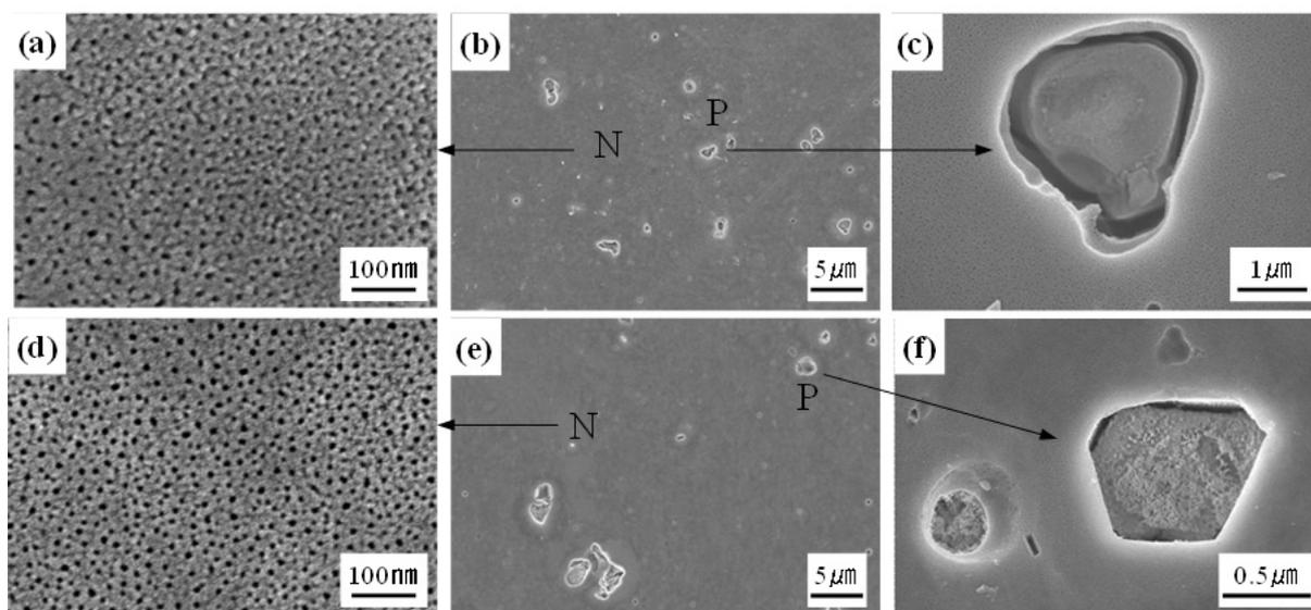
Fig. 3. FE-SEM images of Al-Mg alloy without ECAP (a, b, c) and with (d, e, f) anodized at  $400 \text{ A}\cdot\text{m}^{-2}$  for 40 min.
