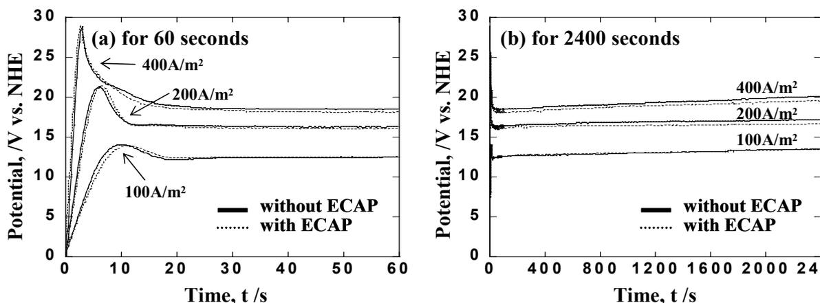
Fig. 2. Time-dependence of anode potential of Al-Mg substrate (a, b) during anodization at various current densities in a solution containing  $1.53 \text{ mol}\cdot\text{L}^{-1}$  of  $\text{H}_2\text{SO}_4$  and  $0.0185 \text{ mol}\cdot\text{L}^{-1}$  of  $\text{Al}_2(\text{SO}_4)_3$  at 293K.
