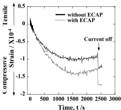
Fig. 7. Time-dependence of strain of Al-Mg alloy substrates during anodization at 400 A·m<sup>-2</sup> in a solution containing 1.53 mol·L<sup>-1</sup> of H<sub>2</sub>SO<sub>4</sub> and 0.0185 mol·L<sup>-1</sup> of Al<sub>2</sub>(SO<sub>4</sub>)<sub>3</sub> at 293K.
