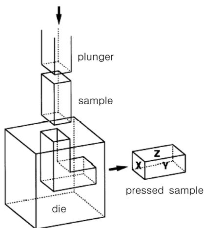
Fig. 1. Schematic diagram of ECAP.
