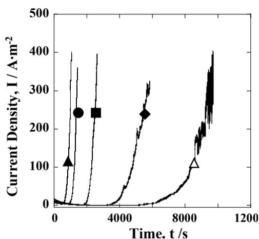
Fig. 5. Effect of annealing on the time-dependence of the anodic current density of Al-Mg alloy anodized at 400 A·m<sup>-2</sup> while kept at constant potential of 1.2V in 0.2 mol·L<sup>-1</sup> of AlCl<sub>3</sub> solution. ▲: annealing-free, ●: 473K, ■: 523K, ◆: 573K, △: without ECAP, ▲●■◆: with ECAP
