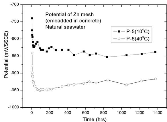
Fig. 10. Potential of Zn-mesh anode at two different temperatures
