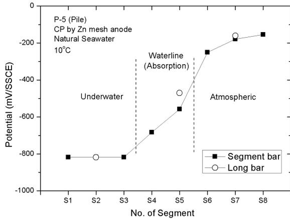
Fig. 7. The potential difference between the segment and the long bars for P-5 specimen
