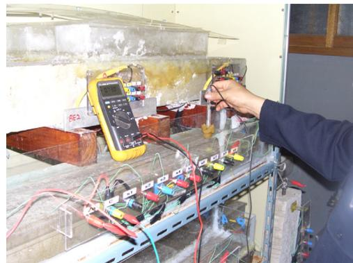
Fig. 3. Potential measurement of a specimen
