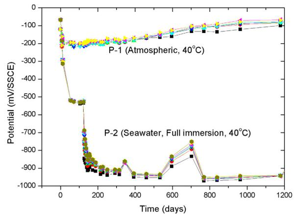
Fig. 4. Potential variation with time of the 8 segments for P-1 & P-2 specimens
