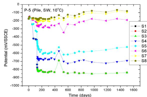
Fig. 5. Potential vs. Time of 8 segments for P-5 specimen
