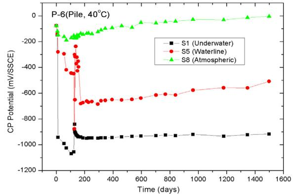
Fig. 8. Potential variations of the long bar for P-6 specimen.
