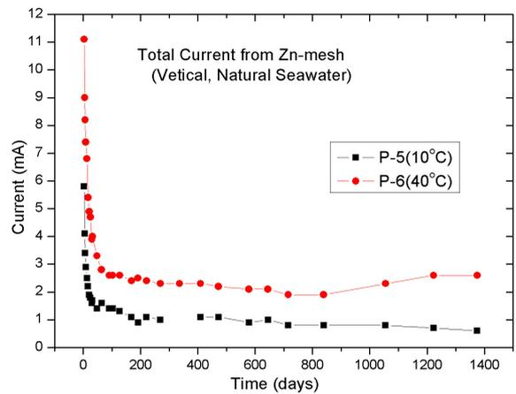
Fig. 9. Total current generated from Zn-mesh anode At two different temperatures
