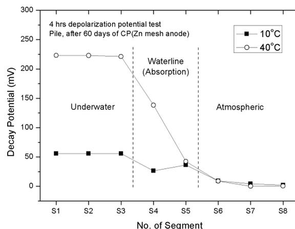
**Fig. 11.** 4 hours depolarization potential after 60 days of cathodic protection by Zn-mesh anode
