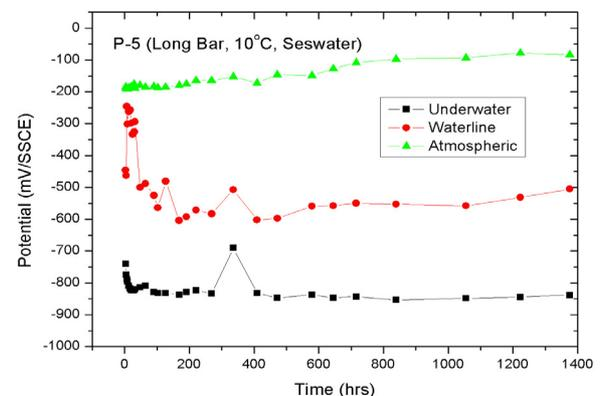
Fig. 6. Potential variations of long bar for P-5 specimen
