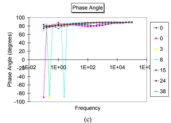
**Fig. 4.** The impedance as a function of frequency for the a) first epoxy-acrylate, b) second epoxy-acrylate and c) automotive reference.
