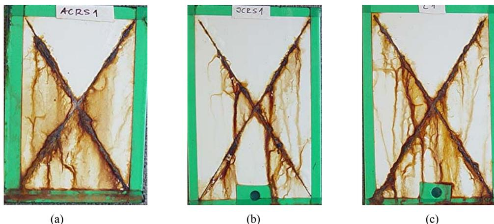
**Fig. 6.** Salt spray test results of CRS panels after 1250 hours a) old epoxy-acrylate, b) new epoxy-acrylate and c) automotive reference.
