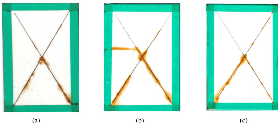
**Fig. 2.** Salt water immersion test results of CRS panels after 7 weeks; a) first epoxy-acrylate, b) second epoxy-acrylate and c) automotive reference.
