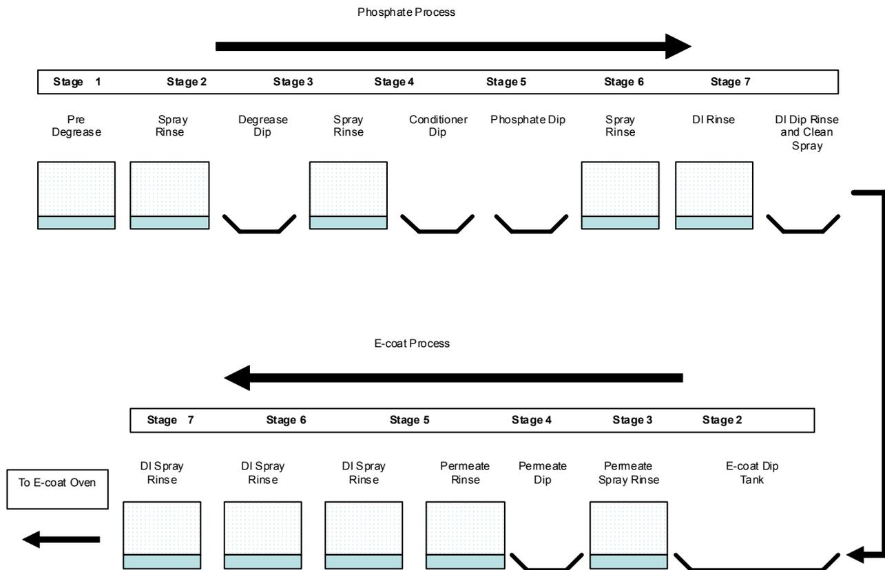
Fig. 1. The pretreatment and e-coating steps of a typical finishing line in the automotive industry.
