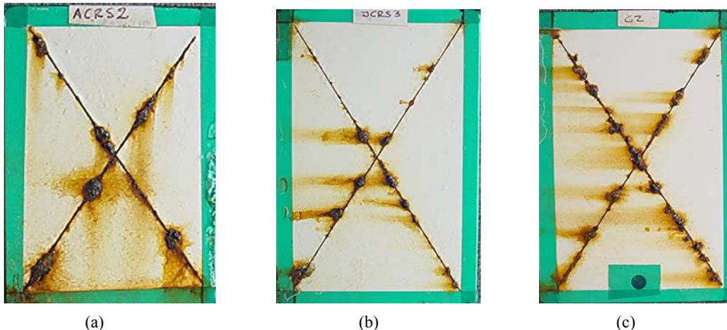
**Fig. 3.** Ford test results of CRS panels after 38 cycles; a) first epoxy-acrylate, b) second epoxy-acrylate and c) automotive reference.
