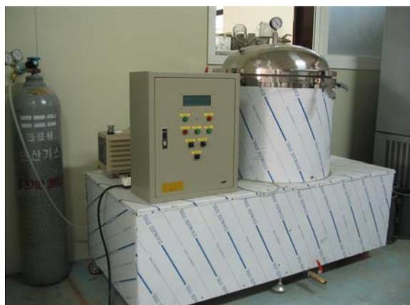
Fig. 2. Accelerated carbonation equipment
