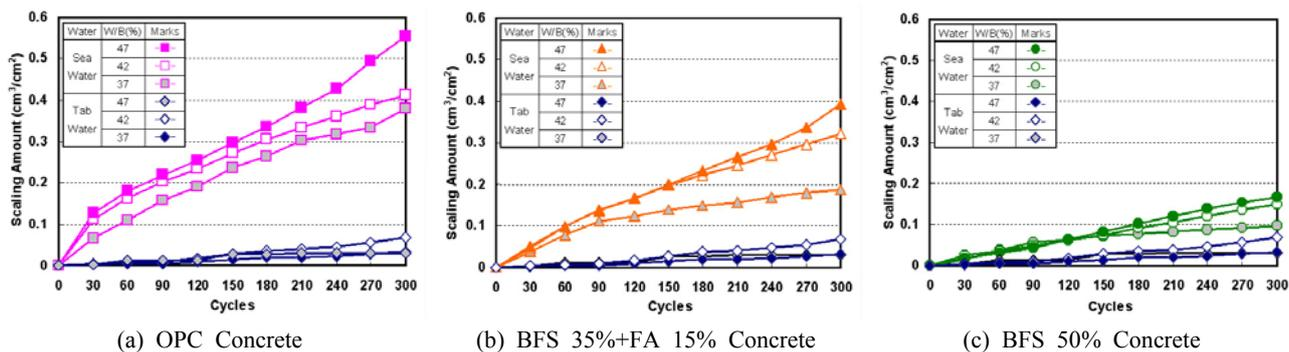
Fig. 5. Surface scaling amount of concrete with binder types
