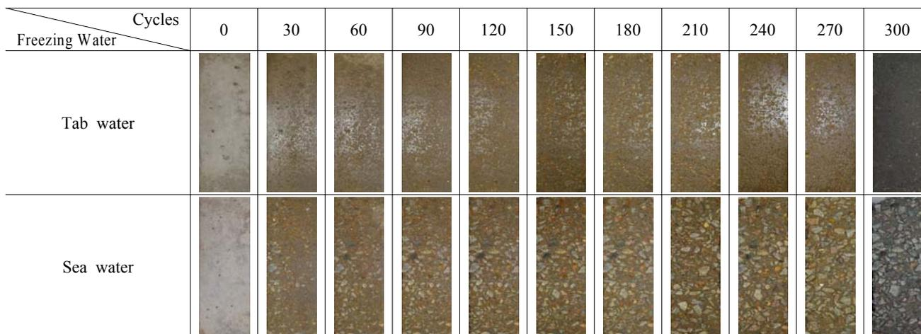
Photo 2. Surface scaling with freezing water (W/B 42% OPC Concrete)
