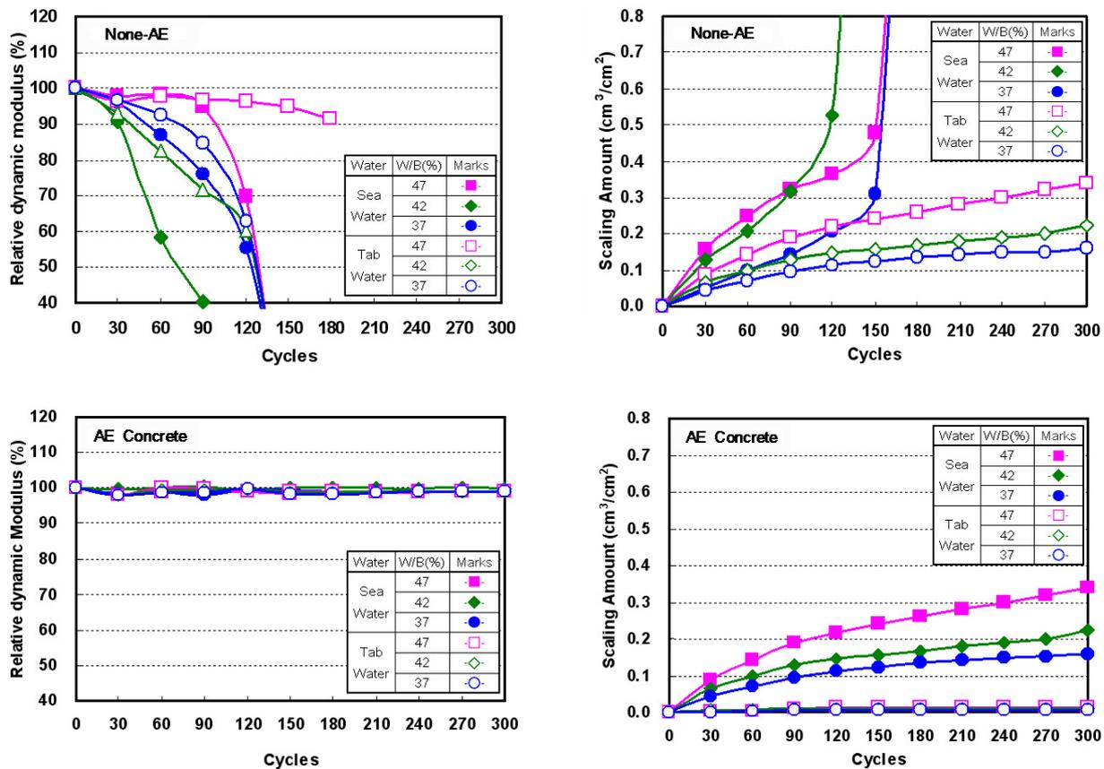
Fig. 2. Relative dynamic modulus and surface scaling amount of None AE Concrete and AE Concrete with freezing-thawing
