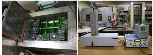
(a) Freezing-thawing testing (b) Evaluation of dynamic elasticity modulus
