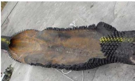
Fig. 6. Ruptured tube appearance after dissection
