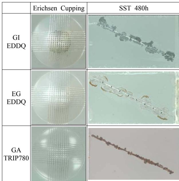
**Fig. 1.** Comparison of Adherence and Corrosion Properties of GI/EG/GA
