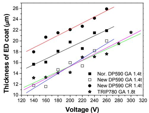
**Fig. 2.** Dependence of thickness of ED coat on ED voltage
