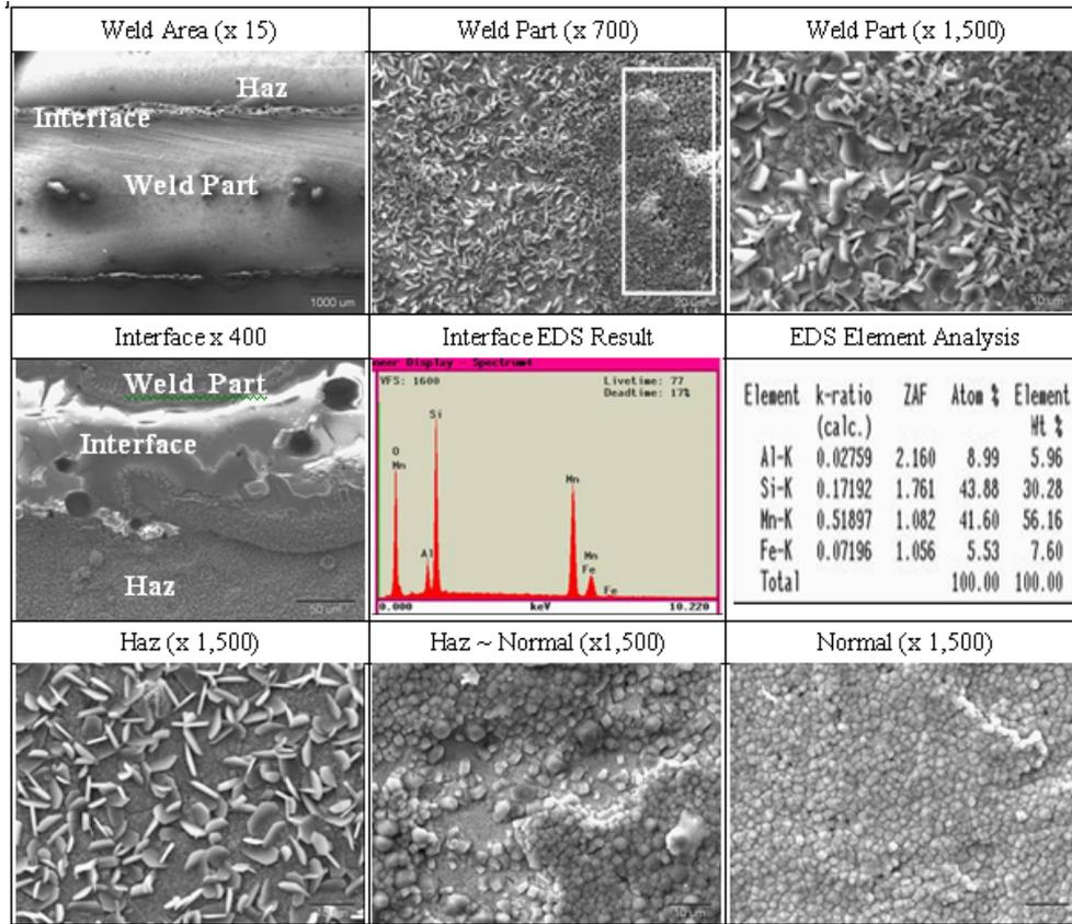
Fig. 4. Phosphate on arc weld area of DP590 CR. Number in ( ) is magnification of SEM.
