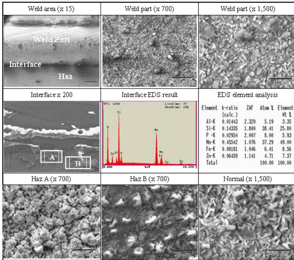
Fig. 6. Phosphate on arc weld area of DP590 GA. Number in ( ) is magnification of SEM.
