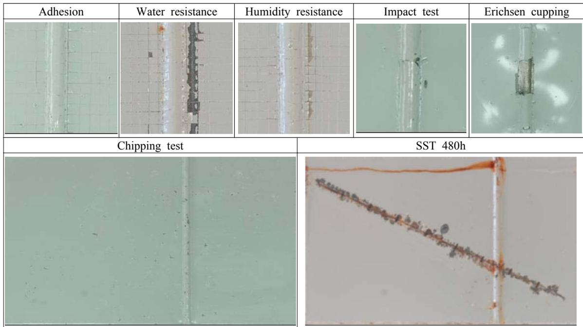
Fig. 7. Paintability in arc weld area of DP590 GA
