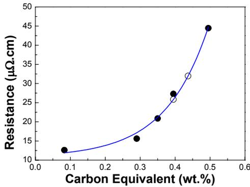
Fig. 3. Relationship between Ceq and Specific resistance of Automotive Steels
