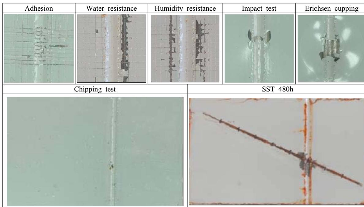
Fig. 5. Paintability in arc weld area of DP590 CR
