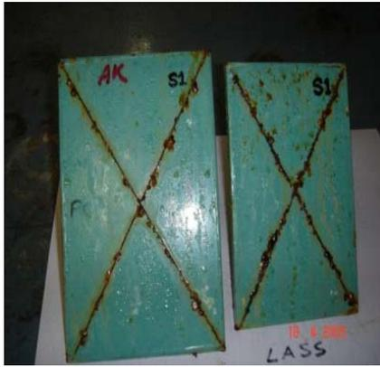
Fig. 4. Rust on PCS & LAS in SO<sub>2</sub>
