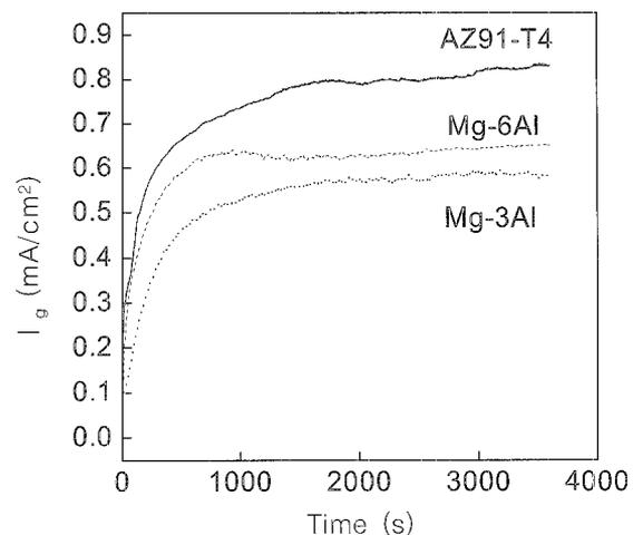
Fig. 5. Galvanic current density in galvanic couples of solid solution alloys and  $Mg_{17}Al_{12}$ (area ratio 10%)
