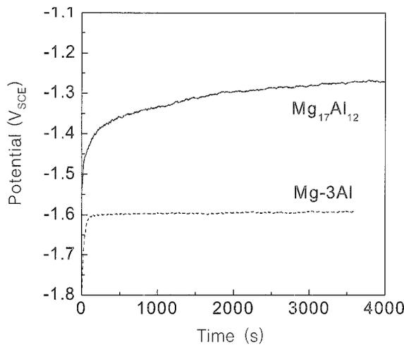
Fig. 2. Variation of the open-circuit potential of  $Mg_{17}Al_{12}$  and Mg-3Al
