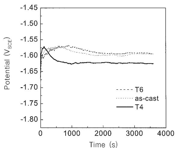
Fig. 1. Variation of the open-circuit potential of AZ91D alloy
