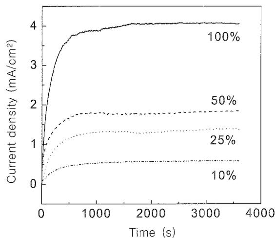
Fig. 3. Variation of galvanic current density with area ratio in Mg-3Al and  $Mg_{17}Al_{12}$  galvanic couple
