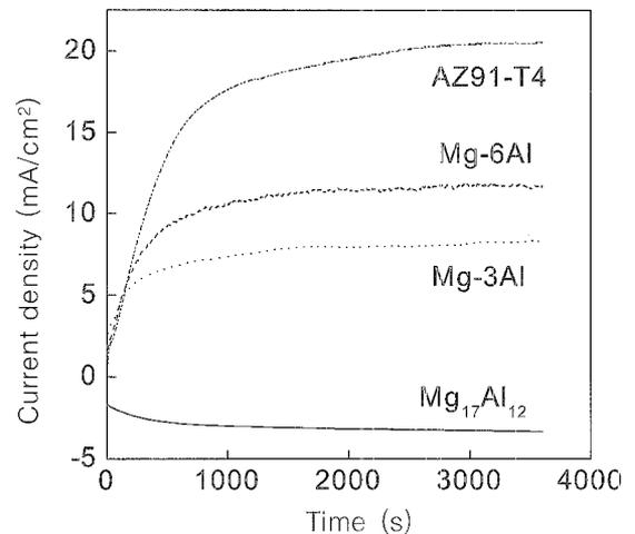
Fig. 4. Current density - time curves for various alloys at an applied potential of -1.57V
