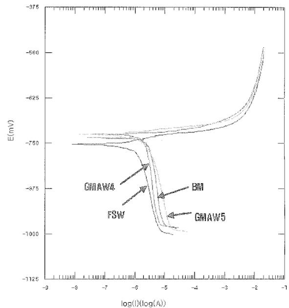
Fig. 3. Comparison of corrosion Rate of each specimens.
