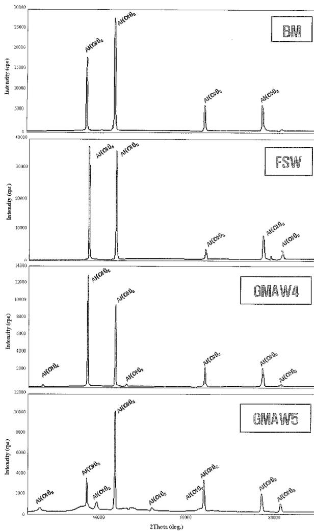
Fig. 7. XRD analysis of each specimen after immersion test.
