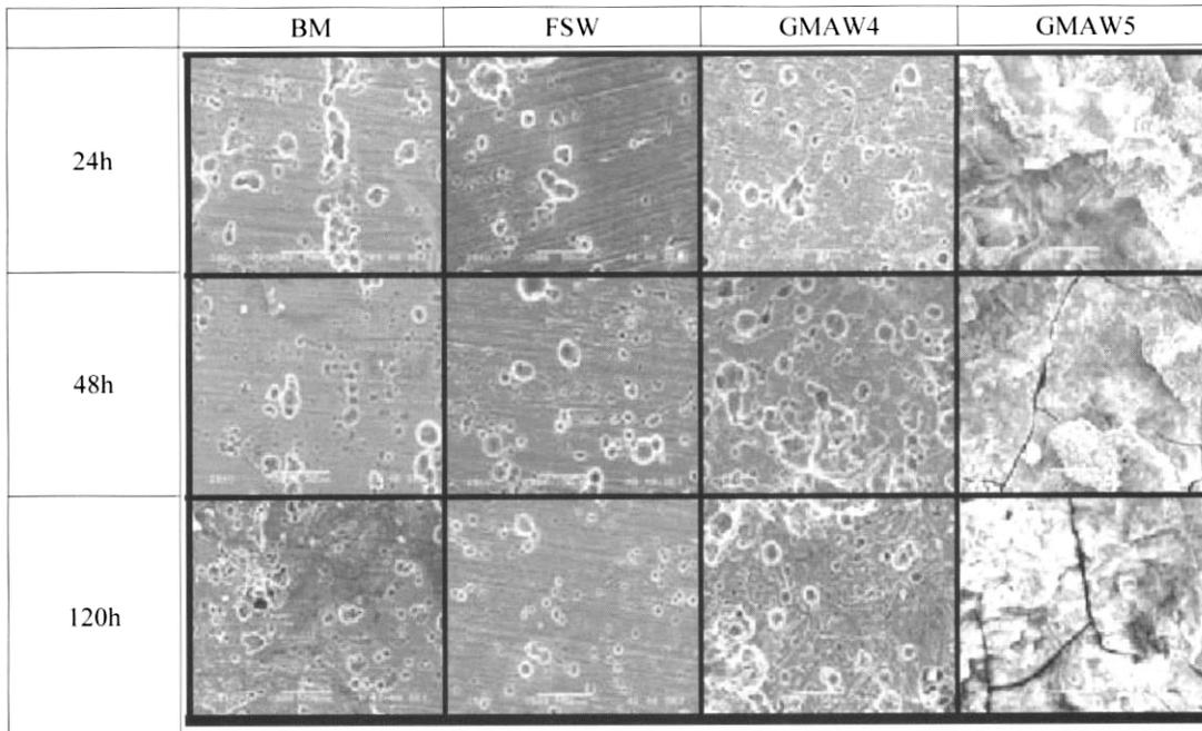
Fig. 5. SEM photos of each specimens after immersion test.
