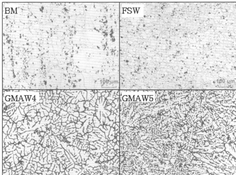
**Fig. 1.** Microstructure of Al 6061 alloy weld metals.
