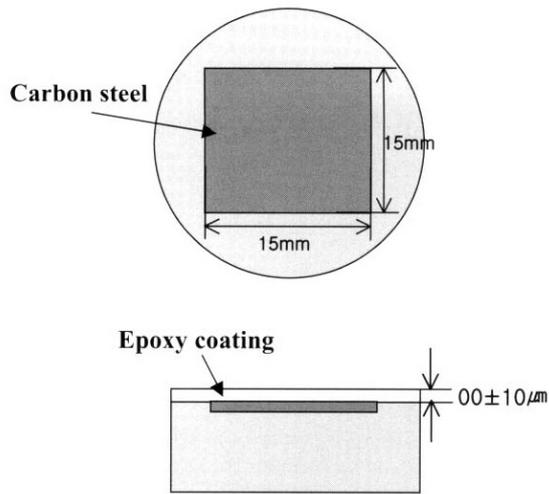
Fig. 1. Schematic diagram of electrochemical impedance cell.
