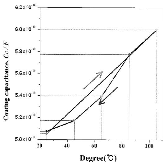
Fig. 4. Reversible change of the coating capacitance values for epoxy coating during thermal cycling.
