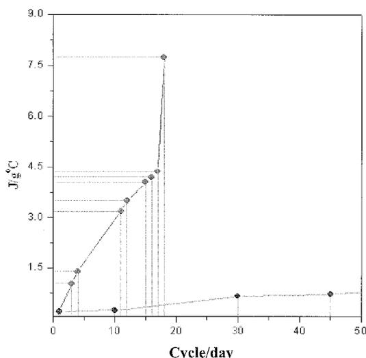
**Fig. 8.** Change of  $\Delta H$  characteristics of epoxy coating during hydrothermal cyclic test and immersion test.
