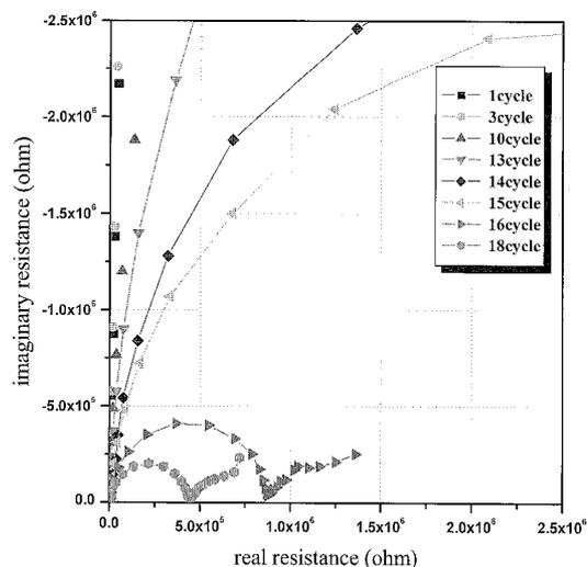
Fig. 6. Nyquist plot for epoxy coating during hygrothermal cyclic test.
