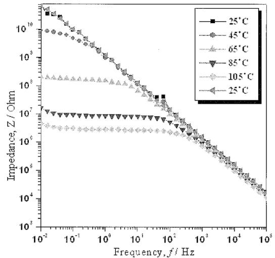
Fig. 3. EIS modulus of epoxy coating at different temperatures.
