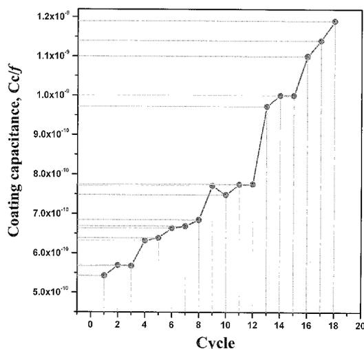
Fig. 7. Change of coating capacitance characteristics of epoxy coating with the number of cycle.
