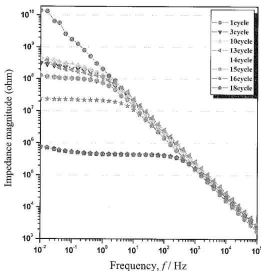
Fig. 5. Change of impedance characteristics for epoxy coating with the number of cycle.
