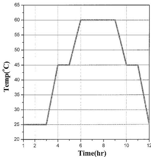
Fig. 2. Diagram of hydrothermal cyclic test process.
