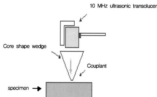
Fig. 3. Concept of measuring impedance
