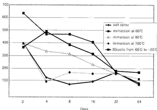
**Fig. 5. Adhesion strength on Steel Specimen**
