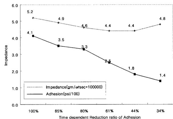
Fig. 11. Relation between adhesion strength and impedance on steel at immersion 80 °C
