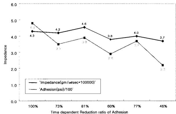
Fig. 10. Relation between adhesion strength and impedance on concrete
