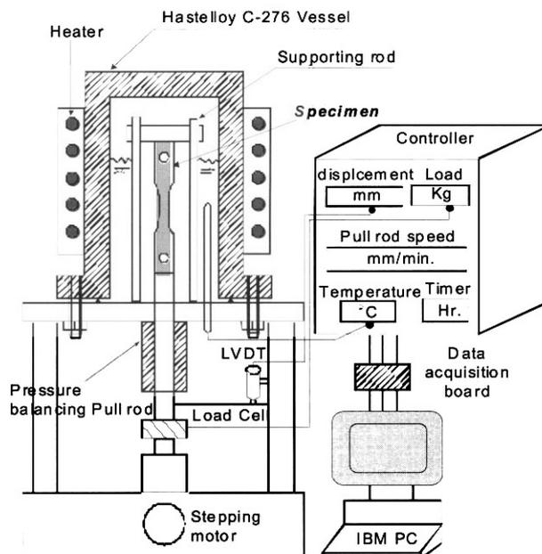
Fig. 2. Schematic of the stress corrosion test system(SSRT)
