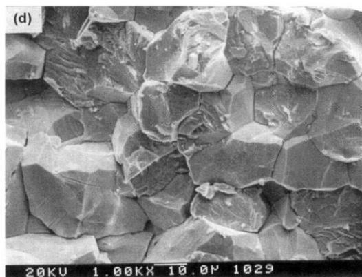
Fig. 10. Severe SCC at pH 10 of alloy 600MA at 340 °C in water containing 10,000 ppm Pb, strain rate is  $1 \times 10^{-7}$ /sec
