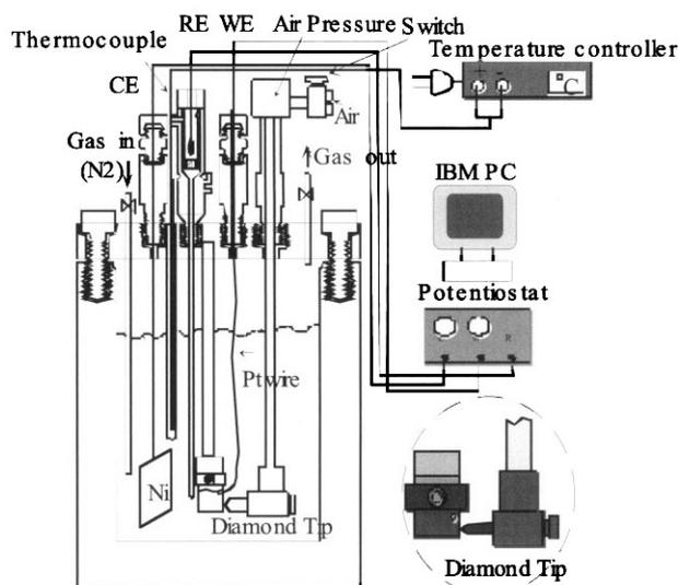
Fig. 1. Schematic of the repassivation rate testing system at a high temperature
