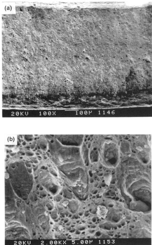
Fig. 9. No SCC at pH 7 of alloy 600MA at 340 °C in water containing 10,000 ppm Pb, strain rate is  $1 \times 10^{-7}$ /sec
