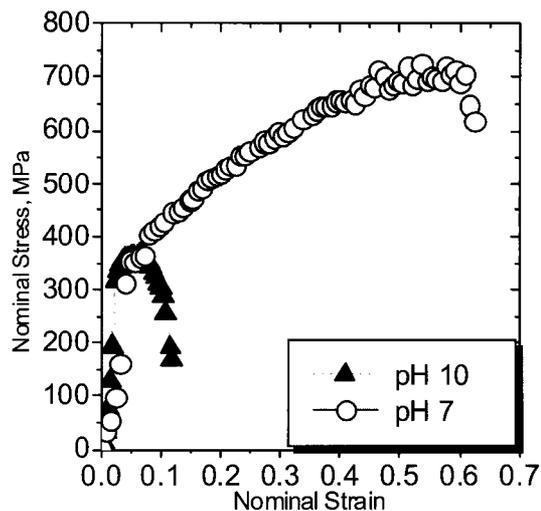
Fig. 11. SCC susceptibility of Alloy 600 MA at different pH conditions at 340 °C in water containing 10,000 ppm Pb, strain rate is  $1 \times 10^{-7}$ /sec.
