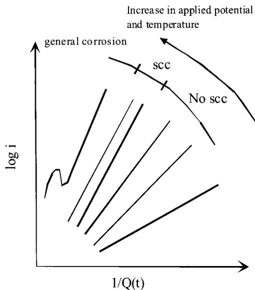
Fig. 5. Stress corrosion tendency for different conditions
