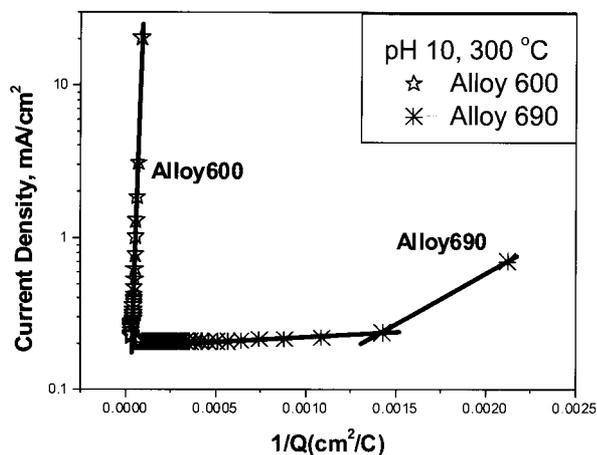
Fig. 8. Current density versus 1/Charge density of the alloys during a repassivation at 300 °C
