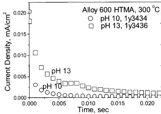
Fig. 4. Comparison of the repassivation behavior of alloy 600 in water at pH 10 and pH 13 at 300 °C.
