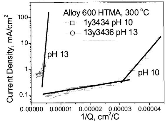
Fig. 6. Effect of the pH on the current transient of alloy 600 at 300 °C
