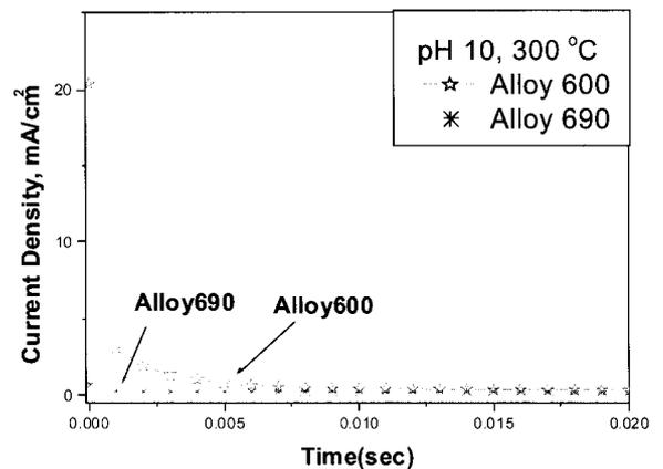
Fig. 7. Effect of the alloy composition on the current transient at 300 °C.
