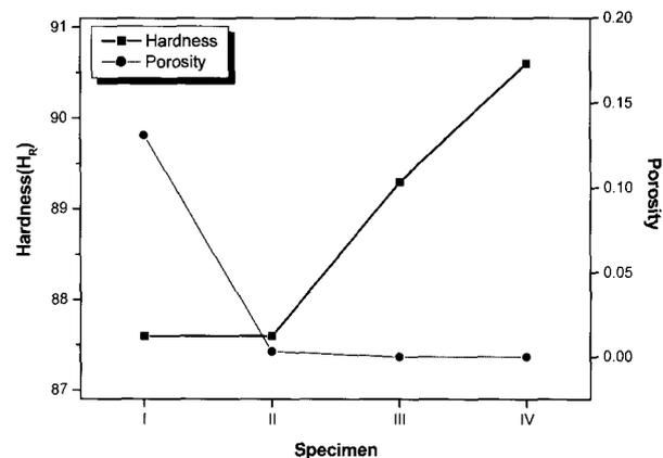
**Fig. 4.** Hardness and porosity of WC-Ti<sub>1-x</sub>Al<sub>x</sub>N coatings; (I) WC-Ti<sub>0.6</sub>Al<sub>0.4</sub>N (II) WC-Ti<sub>0.53</sub>Al<sub>0.47</sub>N (III) WC-Ti<sub>0.5</sub>Al<sub>0.5</sub>N (IV) WC-Ti<sub>0.43</sub>Al<sub>0.57</sub>N.
