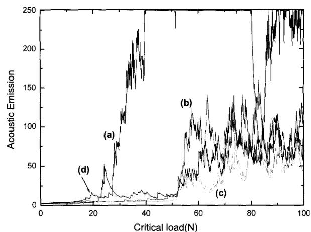
**Fig. 3.** Results of scratch adhesion tests for WC-Ti<sub>1-x</sub>Al<sub>x</sub>N coatings; (a) WC-Ti<sub>0.6</sub>Al<sub>0.4</sub>N (b) WC-Ti<sub>0.53</sub>Al<sub>0.47</sub>N (c) WC-Ti<sub>0.5</sub>Al<sub>0.5</sub>N (d) WC-Ti<sub>0.43</sub>Al<sub>0.57</sub>N.
