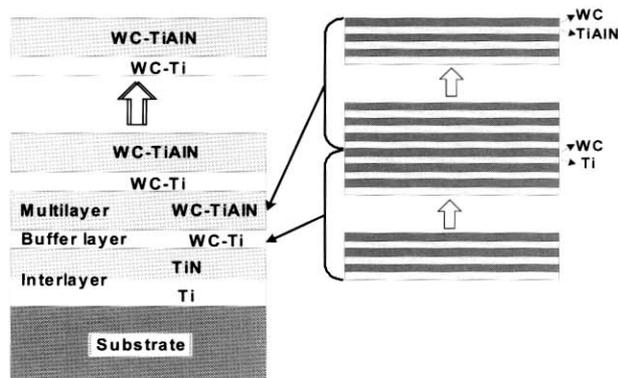
**Fig. 1.** Schematic diagram of the structure of multilayered WC-Ti<sub>1-x</sub>Al<sub>x</sub>N coatings.
