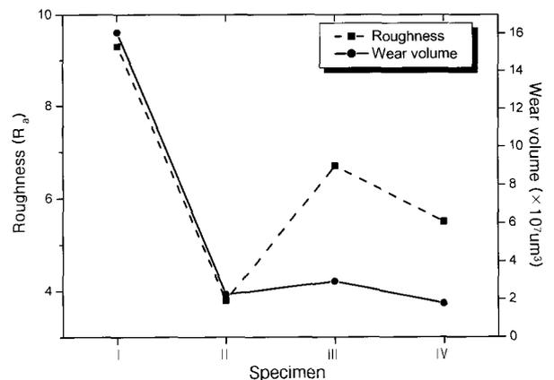
**Fig. 6.** Roughness of coated steels and wear volume of steel balls; (I) WC-Ti<sub>0.6</sub>Al<sub>0.4</sub>N, (II) WC-Ti<sub>0.53</sub>Al<sub>0.47</sub>N, (III) WC-Ti<sub>0.5</sub>Al<sub>0.5</sub>N, (IV) WC-Ti<sub>0.43</sub>Al<sub>0.57</sub>N.
