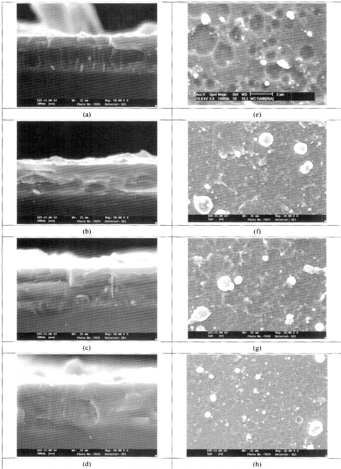
**Fig. 2.** SEM images of a surface and cross-section; (a,e) WC-Ti<sub>0.6</sub>Al<sub>0.4</sub>N (b,f) WC-Ti<sub>0.53</sub>Al<sub>0.47</sub>N (c,g) WC-Ti<sub>0.5</sub>Al<sub>0.5</sub>N (d,h) WC-Ti<sub>0.43</sub>Al<sub>0.57</sub>N.
