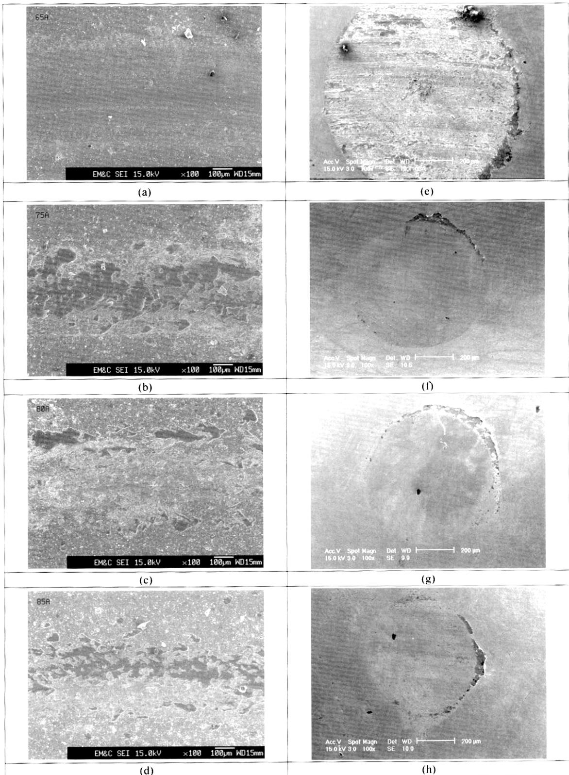
**Fig. 7.** Scanning electron micrographs showing topography of the WC-Ti<sub>1-x</sub>Al<sub>x</sub>N coatings and the wear debris on the wear track; (a-d) the worn surface, and (e-h) the steel ball.
