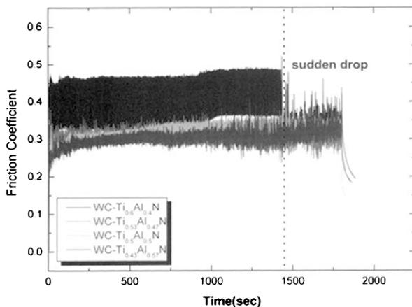
**Fig. 5.** Typical recording of friction coefficient vs. test time when sliding a steel ball against the multilayered coatings; (a) WC-Ti<sub>0.6</sub>Al<sub>0.4</sub>N (b) WC-Ti<sub>0.53</sub>Al<sub>0.47</sub>N (c) WC-Ti<sub>0.5</sub>Al<sub>0.5</sub>N (d) WC-Ti<sub>0.43</sub>Al<sub>0.57</sub>N.
